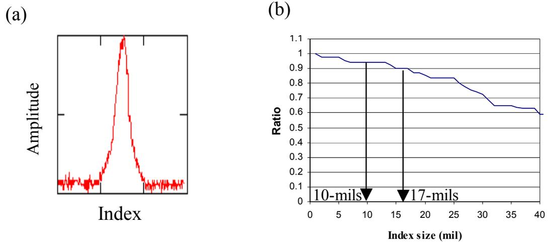
Figure 2. Initial test results showing (a) the eddy current signal amplitude resulting from stepping over the EDM notch at 1-mil index size and (b) the variation of the peak signal amplitude when the index size is increased.
