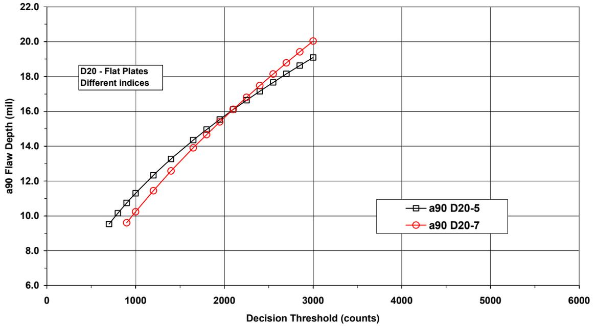
Figure 3. Threshold plots for the D20 coil size with index sizes of 5 and 7 mils.
