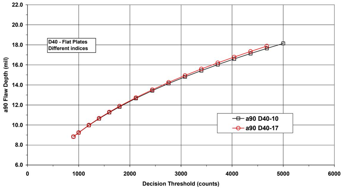
Figure 4. Threshold plots for the D40 coil size with index sizes of 10 and 17 mils.
