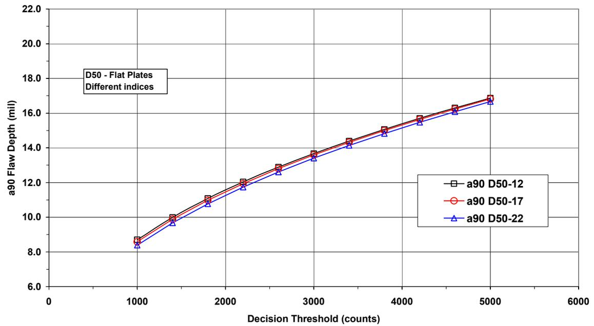
Figure 5. Threshold plots for the D50 coil size with index sizes of 12, 17 and 22 mils.
