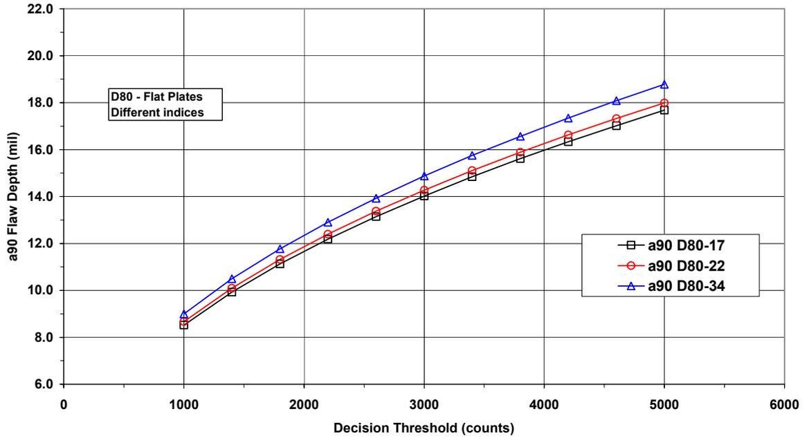
Figure 6. Threshold plots for the D80 coil size with index sizes of 17, 22 and 34 mils.
