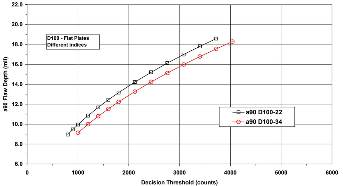
Figure 7. Threshold plots for the D100 coil size with index sizes of 22 and 34 mils.
