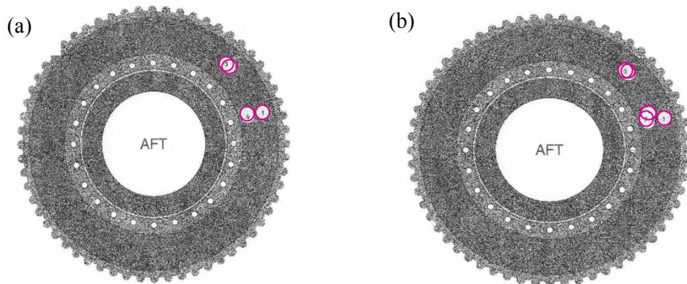
Figure 8. Inspection results of an engine part using D40 coil with (a) regular index size at 10-mils and (b) extended index size of 17-mils. The ratio of time used is 1.7 to 1.
