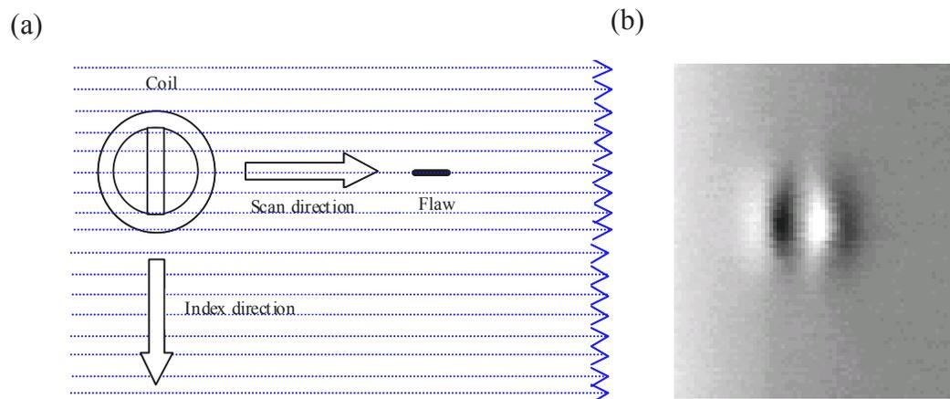
Figure 1. (a) Experimental setup showing the scan and index range over a notched specimen for the initial test and (b) the resultant amplitude image for the area scanned with the brightness proportional to the amplitude.
