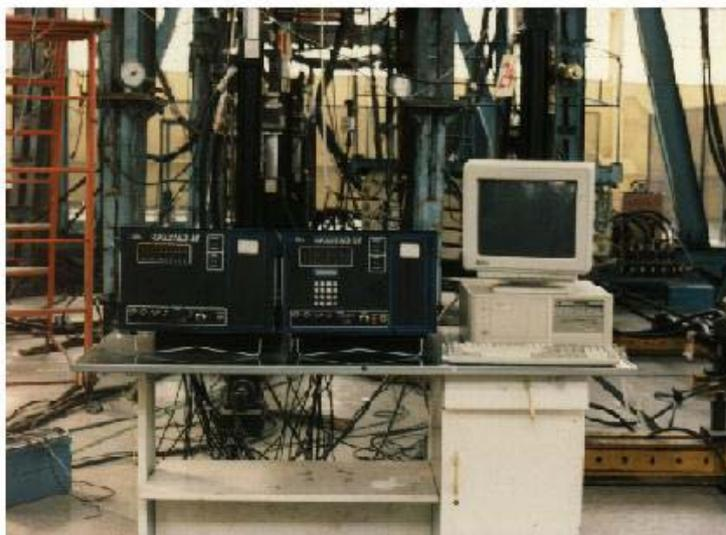
Fig.2 AE test during full-size body fatigue test of a trainer aircraft
