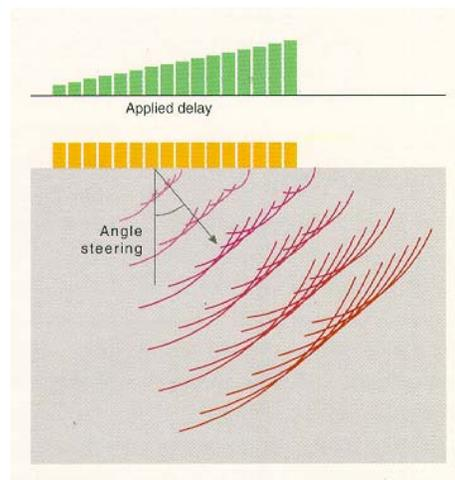
Figure 2: Forming an angle beam with a linear array
