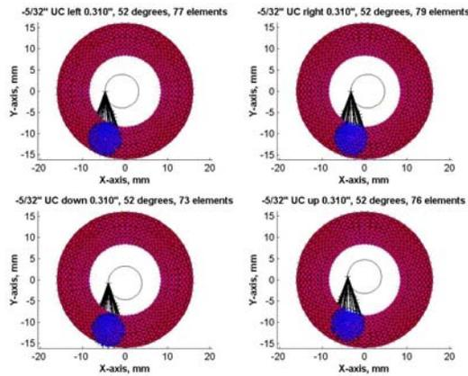
Figure 5: Computer simulation showing array off-center in four directions
