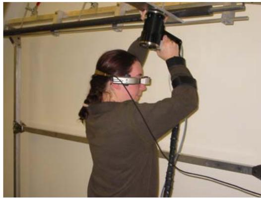
Figure 11: Overhead inspection using the heads-up display
