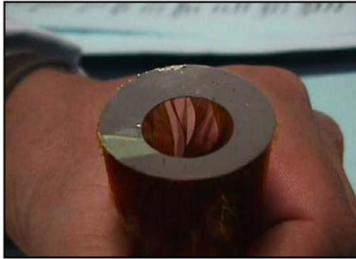
Figure 7: Prototype conical matrix array probe
