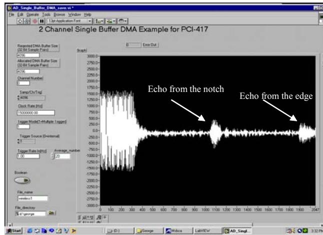
FIGURE 11 - Wireless inspection waveform of the of the 12mm long 50% through wall notch in a 0.8mm thick aluminium plate 26.5mm away from the sensor
