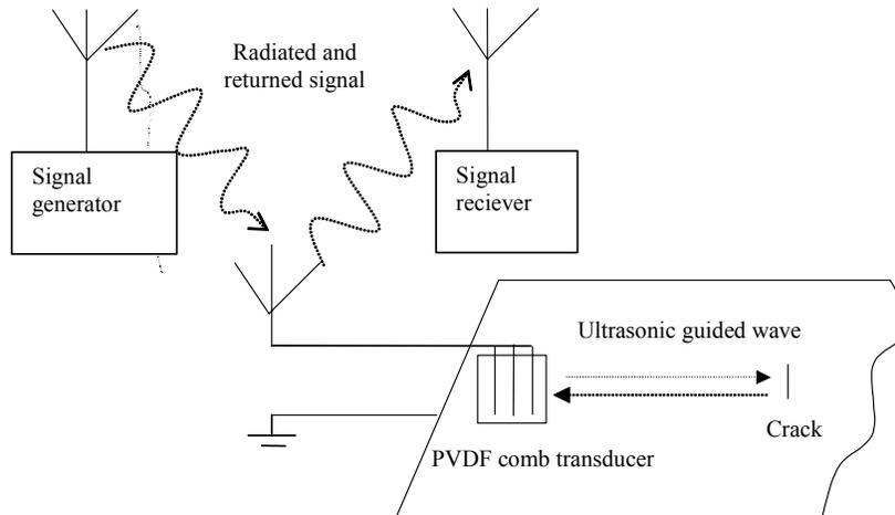
FIGURE 1 - The schematic view of wireless inspection system for crack detection.
