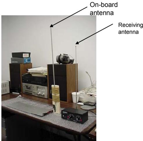
FIGURE 8 - Semi-wireless inspection system setup.
