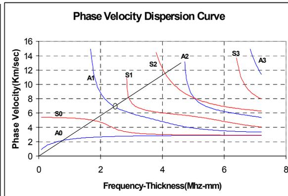
FIGURE 4 - The Group velocity dispersion curve for an aluminum plate (0.8mm).
