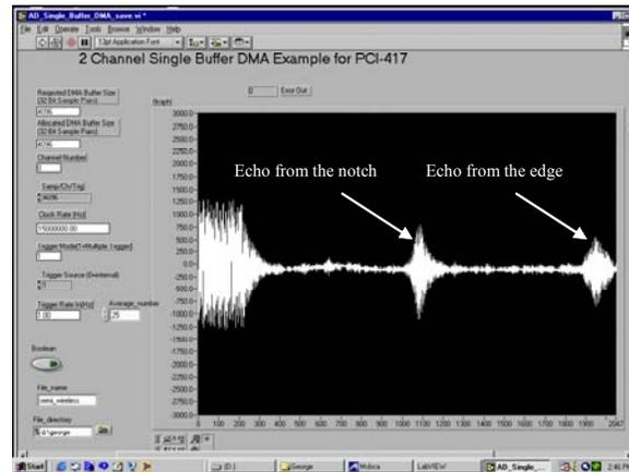
FIGURE 9 - Semi-wireless inspection results of the of the 12mm long 50% through wall notch in a 0.8mm thick aluminium plate 26.5mm away from the sensor
