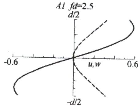
FIGURE 3 - Wave structure for  $A_1$  mode of an aluminum plate for  $fd = 2.5$ . Solid curve denotes the in-plane displacement and dashed curve is the out-plane displacement
