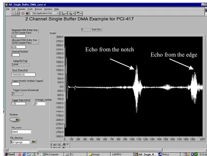
FIGURE 7 - Wired inspection waveform of the 12mm long 50% through wall notch in a 0.8mm thick aluminum plate 26.5mm away from the sensor
