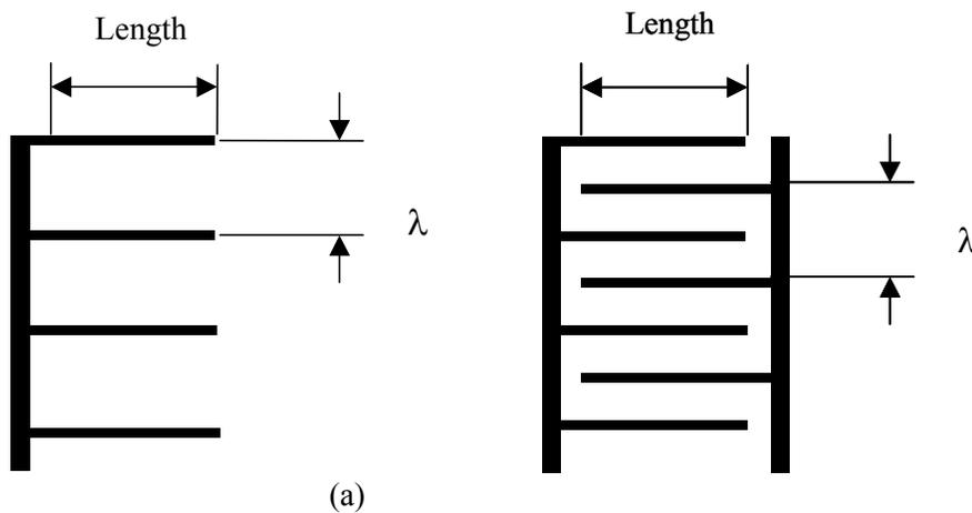
FIGURE 6 - Electrode pattern of PVDF guided wave sensors. (a) The comb pattern. (b) Inter-digital pattern.
