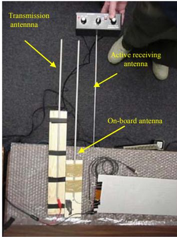
FIGURE 10 - Wireless inspection system setup
