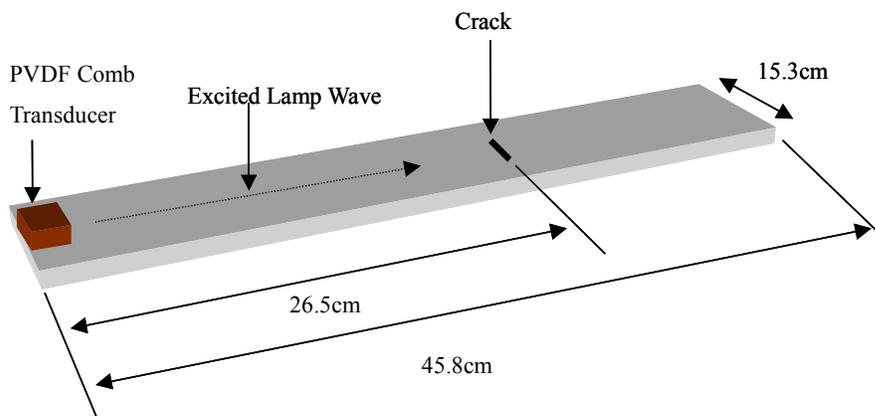
FIGURE 2 - Test specimen with a PVDF comb transducer bonded on the aluminium plate.
