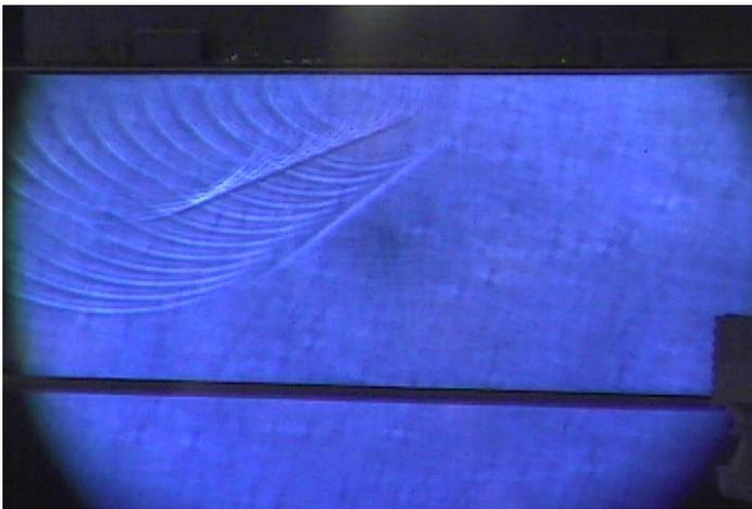
**Figure 6 7.5MHz 60 element probe. Plane wavefront constructed with 12 elements with a 2mm pitch between active elements (no refracting wedge).**
