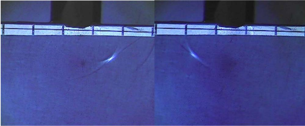
**Figure 5 10MHz 32 element probe. Images show a beam both focused and angled. On the left the beam is focused at 25mm sound path and angled at  $45^\circ$  for the shear mode while on the right the beam is focused at 25mm and angled at  $-45^\circ$  in shear mode. Markers on an acetate overlay indicate 1cm intervals.**
