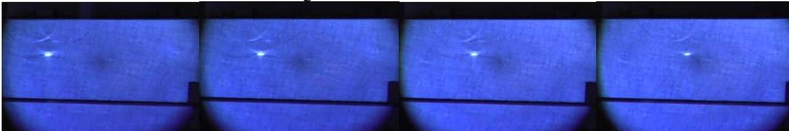
**Images indicate a focused normal beam with the compression mode focused at 15mm in glass and imaged at the focal point. 12 elements are used in the focal laws of a 7.5MHz 60-element probe. The image on the left uses element number 5 as the start element of the 12 and each image then steps the focal law 5 elements further. Images indicate elements 5-16, 10-21, 15-26 and 20-31**
