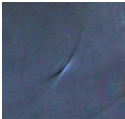
**Figure 9** Raw image of a pulse from a 31 element focal law at 50° focused at 25mm. (7.5MHz 60-element probe with a 33° refracting wedge).
