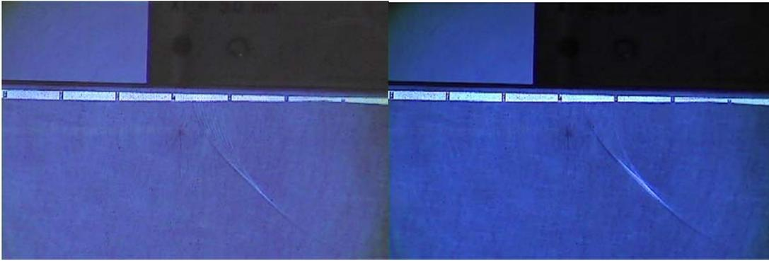
**Figure 7** Image on the left is a 45 refracted plane wavefront (unfocused) using 8 elements and an “aperture” of 16mm. On the right the same plane wavefront is made using 16 elements (7.5MHz 60 element probe).
