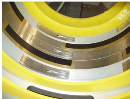
Fig. 6: 6 probes; 4 blocks per probes, 32 elements per block
