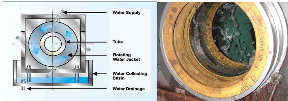
Fig. 5: Rotating water ring with rubber sealings
