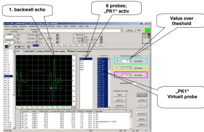
Fig. 9: Operator menu for calibration “virtuel probe”
