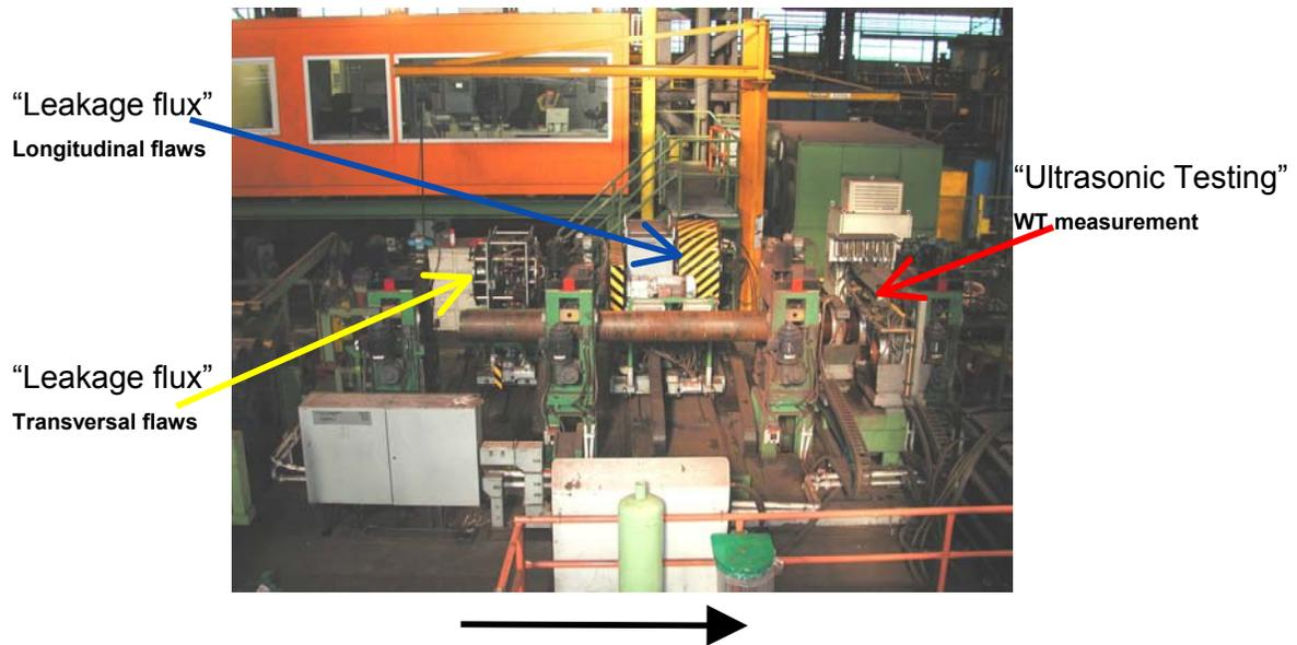
Fig 1: testing machine, overview
