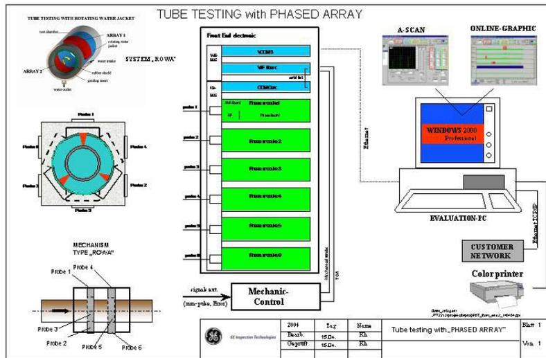
Fig. 3: Schematic Diagram wall thickness measurement
