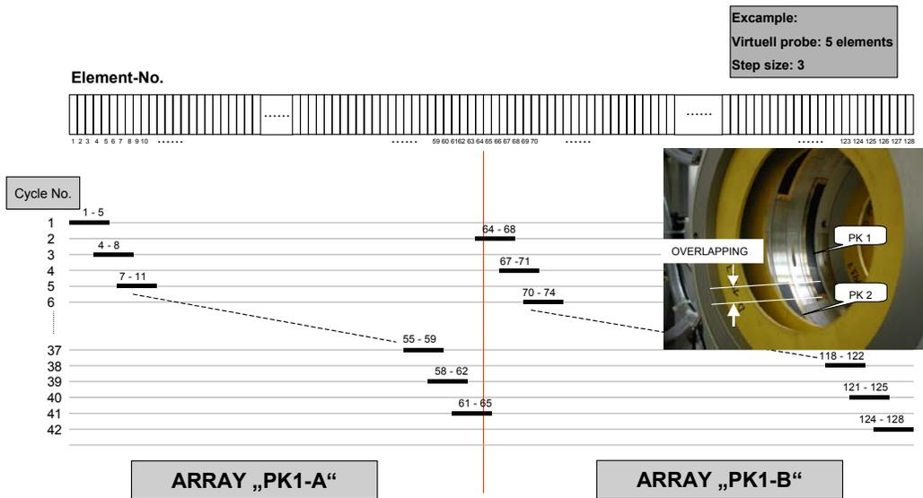
Fig. 7: Cycle diagram; bisection in two Array groups
