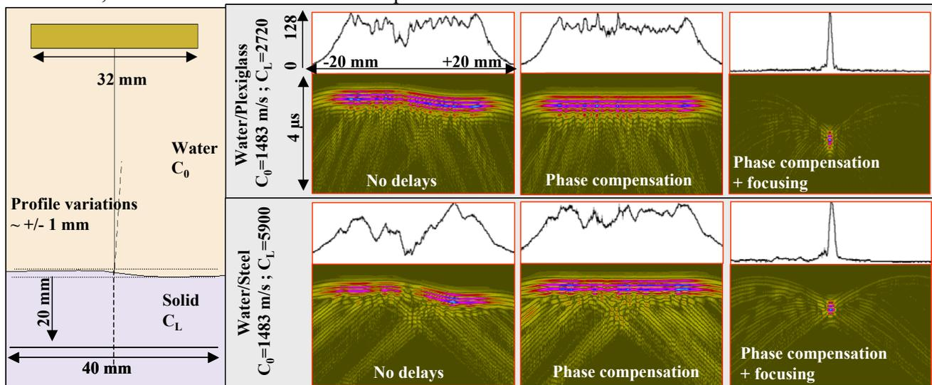
Figure 4: Simulation of phase aberration effects due to an irregular geometry and their compensation using a linear array with adapted delay laws
