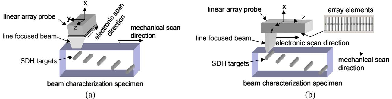
Figure 2. Linear array transducer orientation relative to the SDH characterization block. (a) transducer oriented with the active (focusing) direction parallel to the SDH axis (beam width  $\approx$  element length) (b) transducer oriented with the focusing direction perpendicular to the SDH axis.
