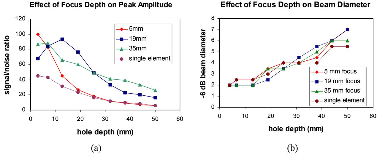
Figure 4 Comparison between a lateral oriented linear array and conventional transducer response to SDH targets: (a) Variation in peak amplitude with SDH depth. (b) variation in -6 dB beam diameter.
