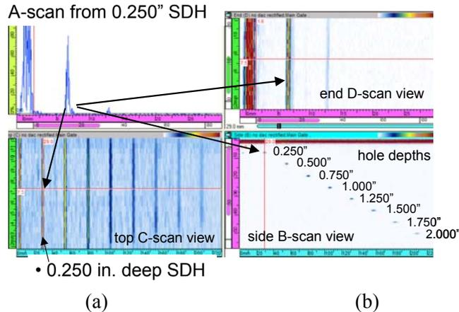
Figure 1. Beam profile characterization for a 10MHz conventional transducer. (a) A-scan reflection from 0.020” SDH and top view C-scan from ultrasonic beam profile characterization block. (b) simulated side and end views of the block cross-section created from A-scan data.
