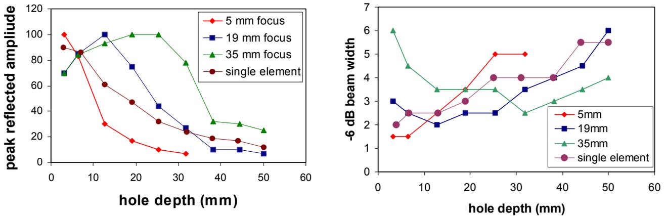
Figure 5 Comparison between a normal orientation linear array and conventional transducer response to SDH targets: (a) Variation in peak amplitude with SDH depth. (b) variation in  $-6$  dB beam diameter. .
