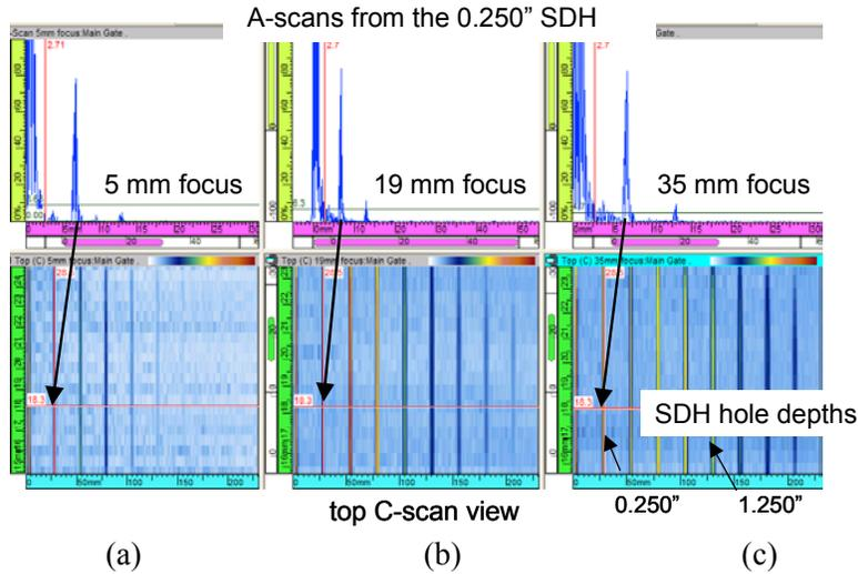
Figure 3. Representative A-scan from 0.250” deep SDH and C-scan images of entire SDH transducer characterization block. Scans were conducted using the linear array in the lateral scanning orientation with the active focusing direction parallel to the SDH axis. Focus depths: (a) 5mm (b) 19mm (c) 35 mm.
