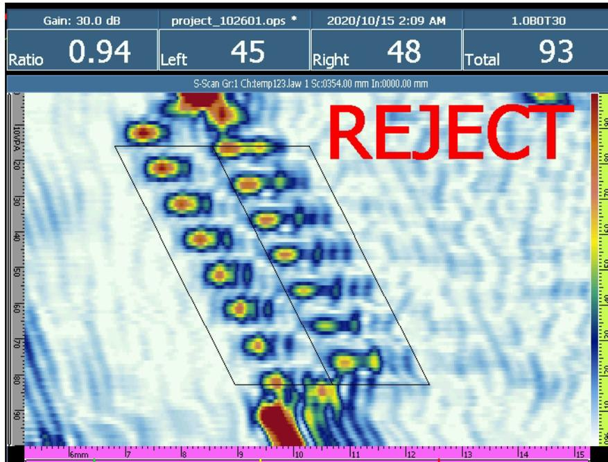
Figure 5: S Scan of a Bad Part with a 90-degree Threading Offset
