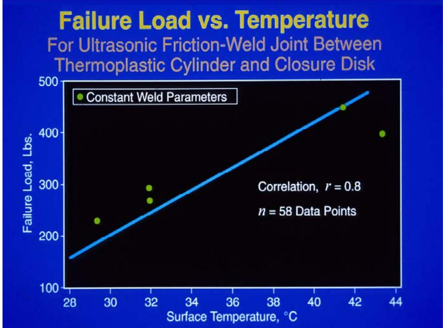
Figure 2. Correlation of disk weld-joint failure load with surface temperature measured by IR 11 seconds after weld completion. Note the scatter among the four data points, shown as green dots,
