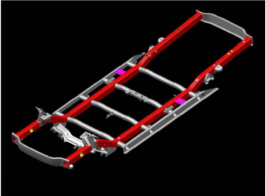
Figure 6. *The all metal CCV frame to which the body is bonded and mechanically fastened*
