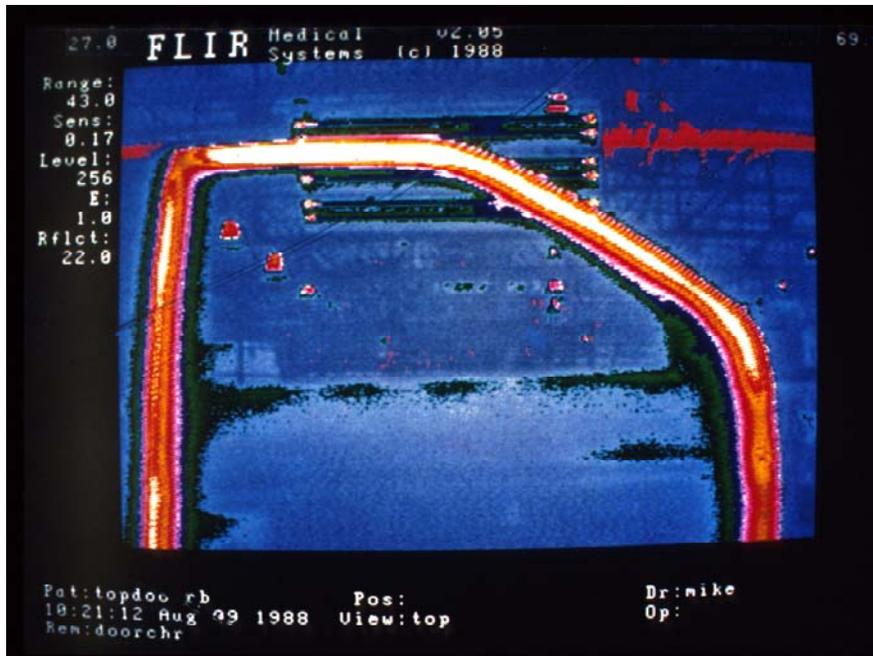
Figure 7. *The thermal image of a vehicle front door after the adhesively bonded hem flange has been thermally cured to a partially cured “green state” by inductive heating*
