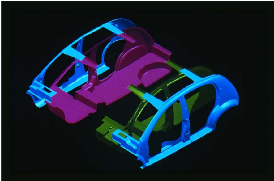
Figure 5. The four major injection-molded, thermoplastic CCV body parts before assembly
