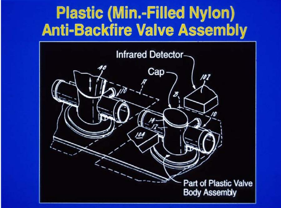
Figure 1. A thermoplastic component being vibration welded at left and monitored for IR emission at right. Note vertical arrow indicating the motion of the 20 kHz ultrasonic horn pressed atop the assembly at left and the detectors to monitor the welded region of the assembly at right.
