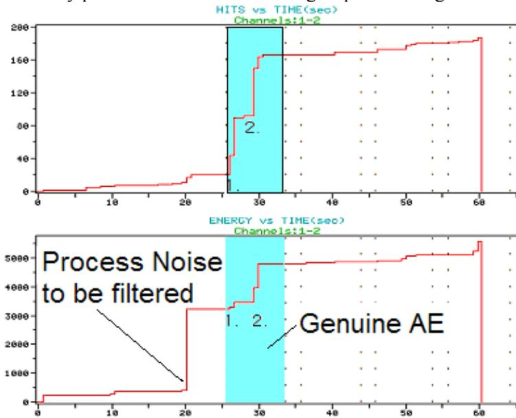
Figure 5: Hit and energy evolution versus time at position 1.
