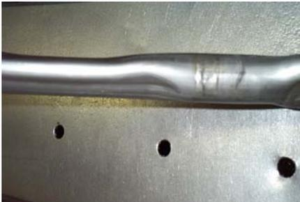
Figure 8: Picture of cracked tube.
