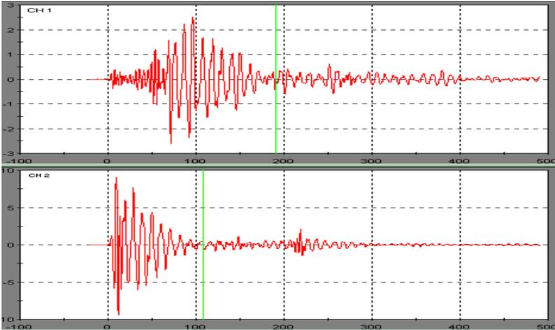
Figure 1: example of AE hits
