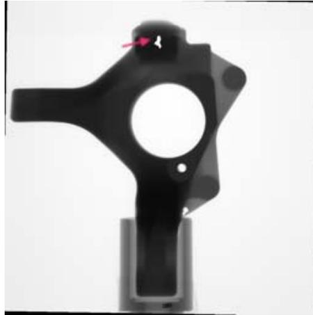
Shrinkage cavity (segmented)
