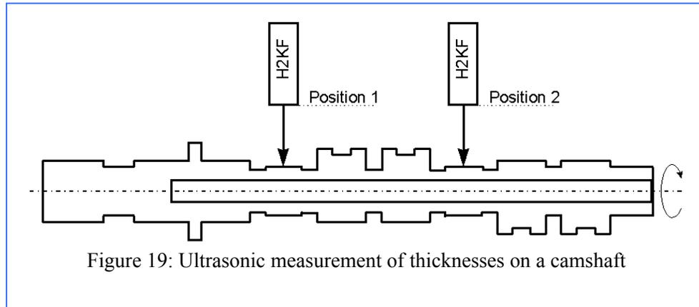
The recommended solution is to measure the wall thickness on the bearing points. The simple, annular geometry of these points enable the shaft to be tested in the casted state. Further processing actions on any defective parts can thus be excluded.
