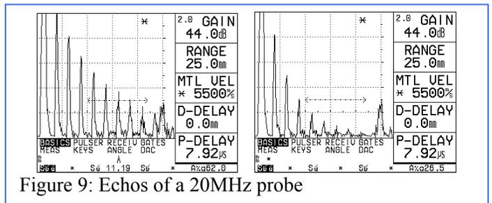
Figure 9: Echos of a 20MHz probe
