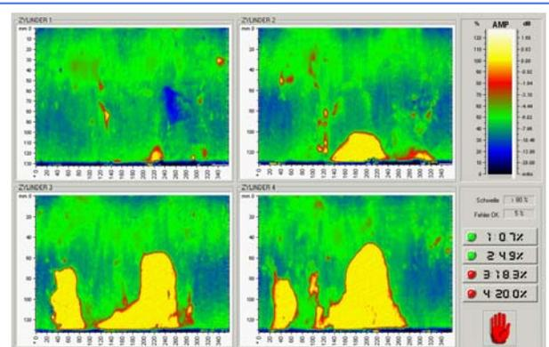
Figure 18: C-scan-plots of 4 cylinders
