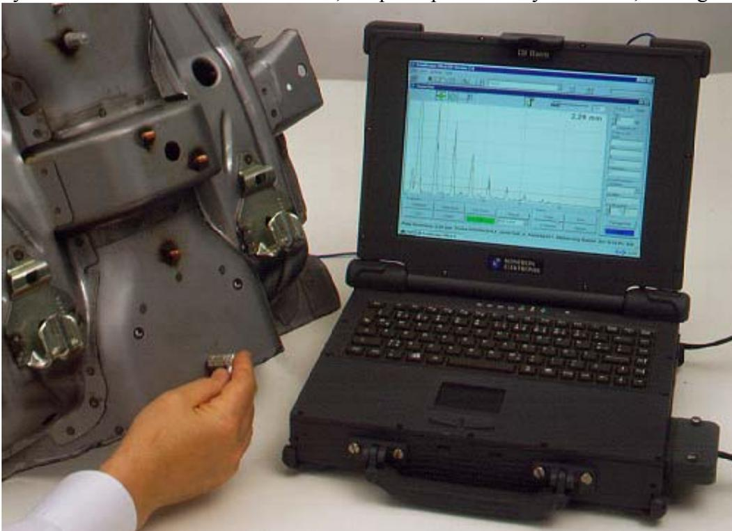
Figure 1: Spot Weld Inspection
