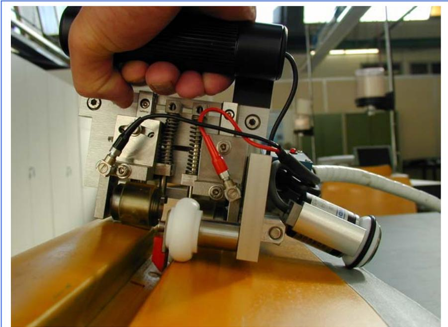
Figure 4: The roller probe setup for the laser weld inspection
