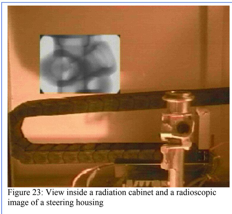
Figure 23: View inside a radiation cabinet and a radioscopic image of a steering housing
