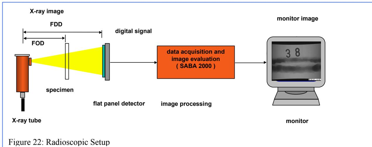
Figure 22: Radioscopic Setup
