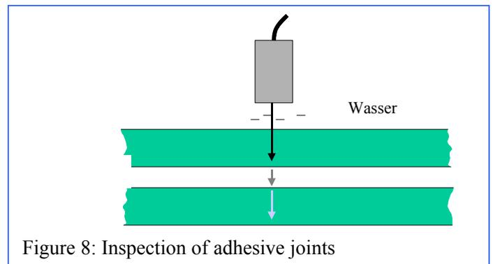
Figure 8: Inspection of adhesive joints
