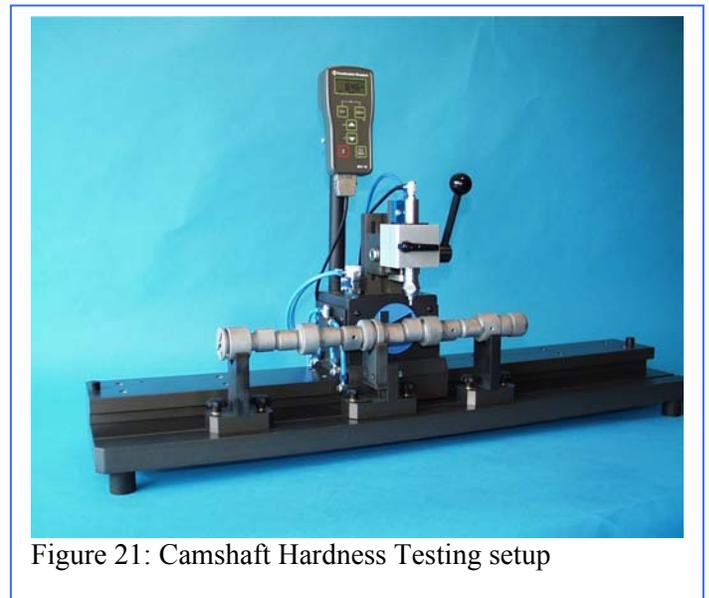
Figure 21: Camshaft Hardness Testing setup
