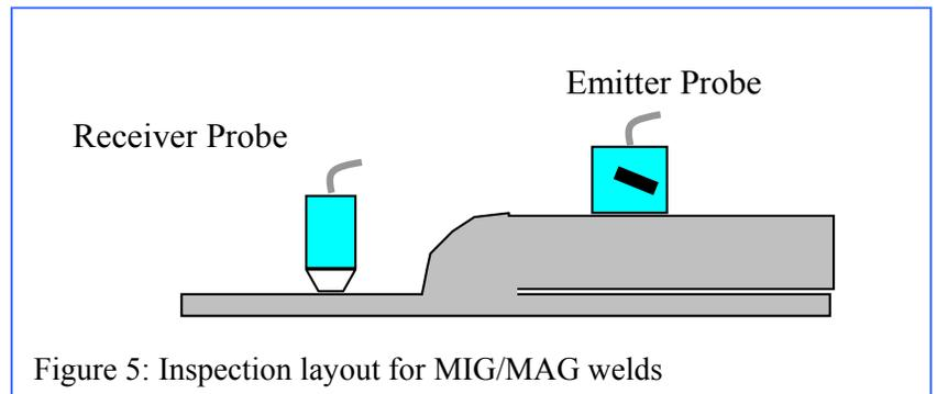
Figure 5: Inspection layout for MIG/MAG welds
