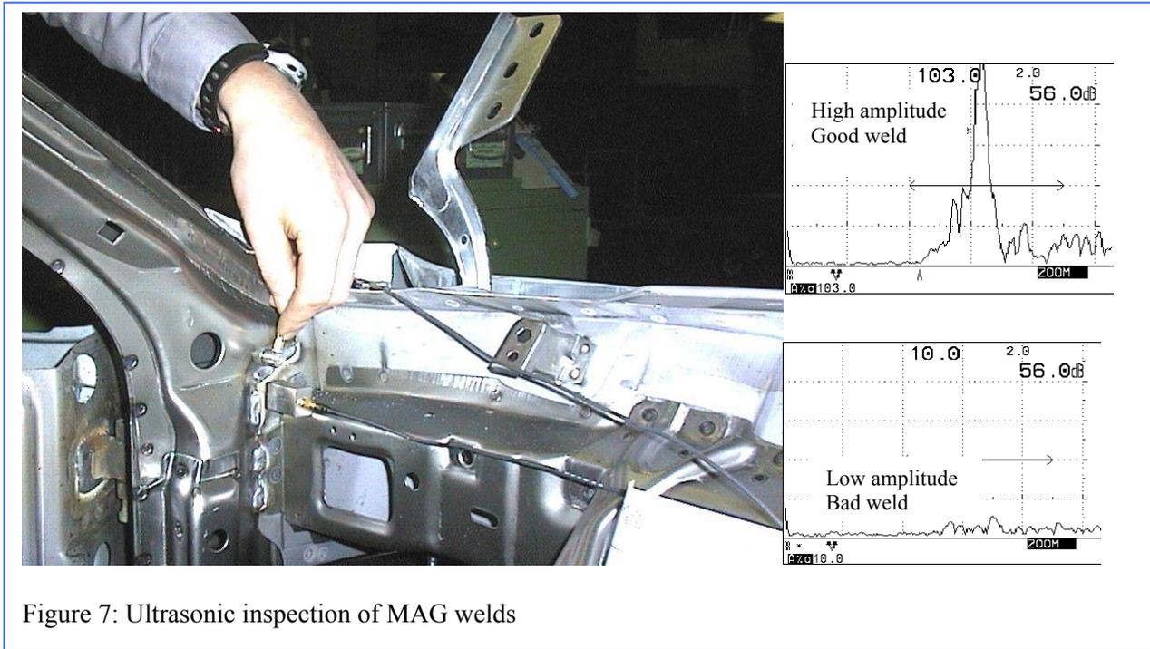
Figure 7: Ultrasonic inspection of MAG welds
