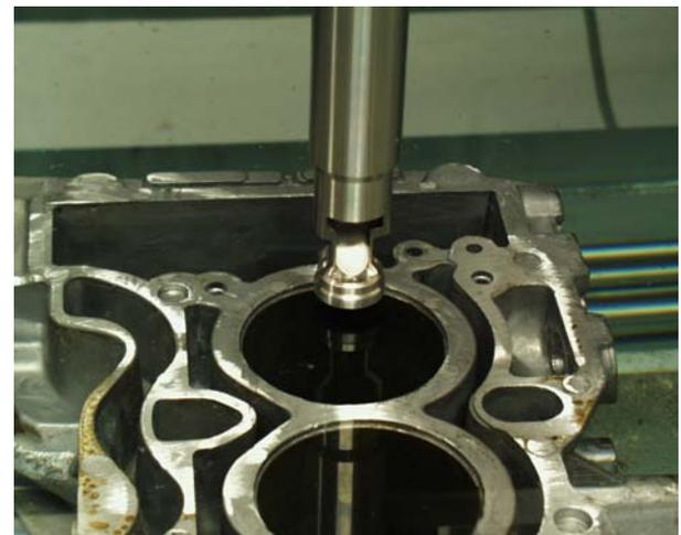
Figure 17: The motor block and the ultrasonic probe with deflection mirror
