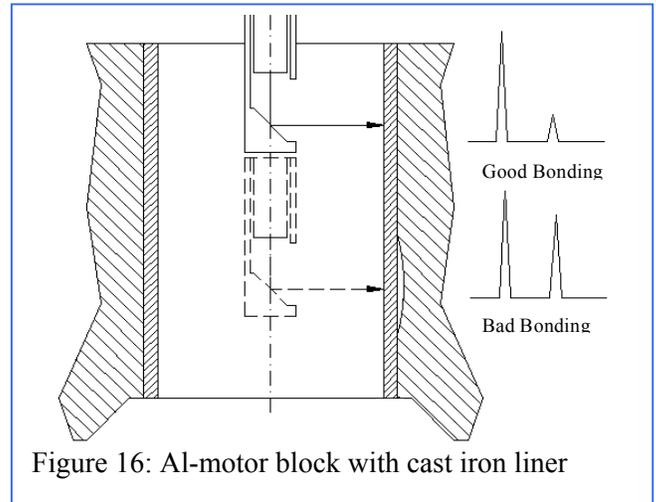
Figure 16: Al-motor block with cast iron liner
