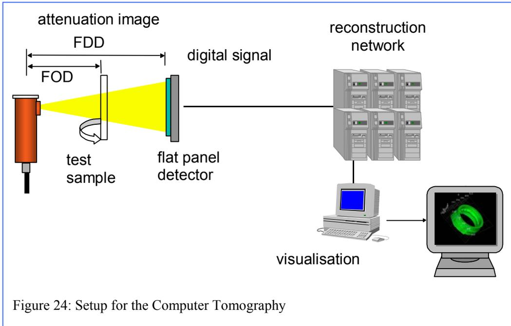
The complete information however can be obtained using tomographic methods. Here, the test sample is rotated in the X-ray beam, see Figure 24, and the intersections of the object or even three dimensional images are obtained by means of a computer reconstruction.
