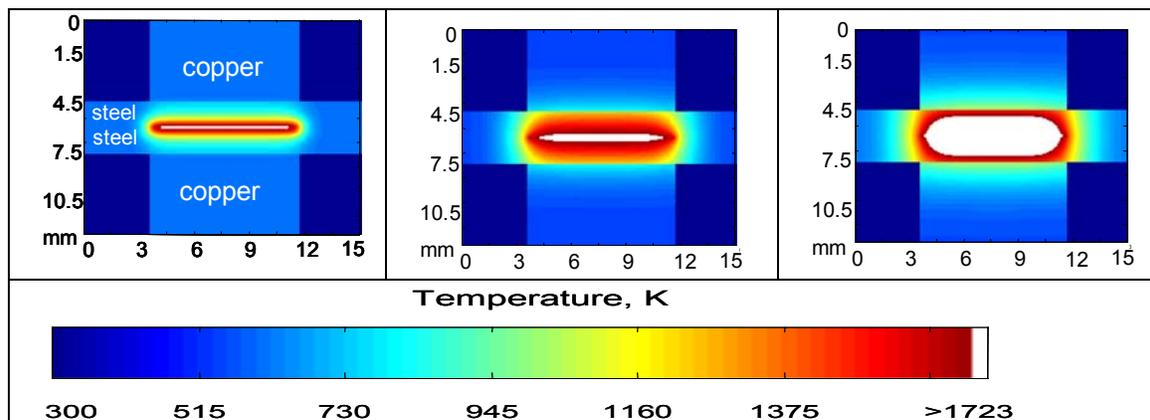
Figure 2. Three samples of temperature distribution in the spot weld during 12 cycles 60 Hz welding procedure. Left picture – second cycle of welding, middle – sixth, right – eleventh cycle.
