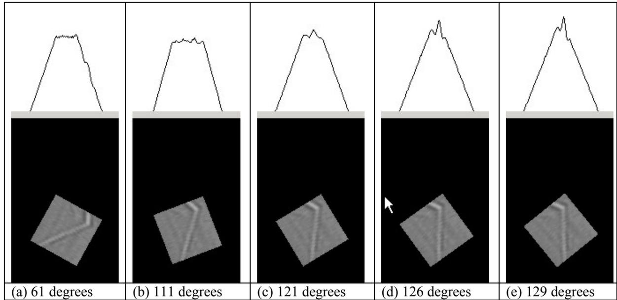
Figure 7. Rotated image segment (bottom) and corresponding normalized projections of the image on the horizontal axis (top).
