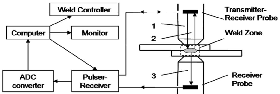
Figure 1. Schematic view of the experimental setup. 1 – incident wave, 2 – reflected wave, 3 – transmitted wave.
