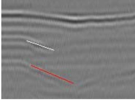
Figure 9. Signature of the weld with the segments of lines located using Radon transform technique.
