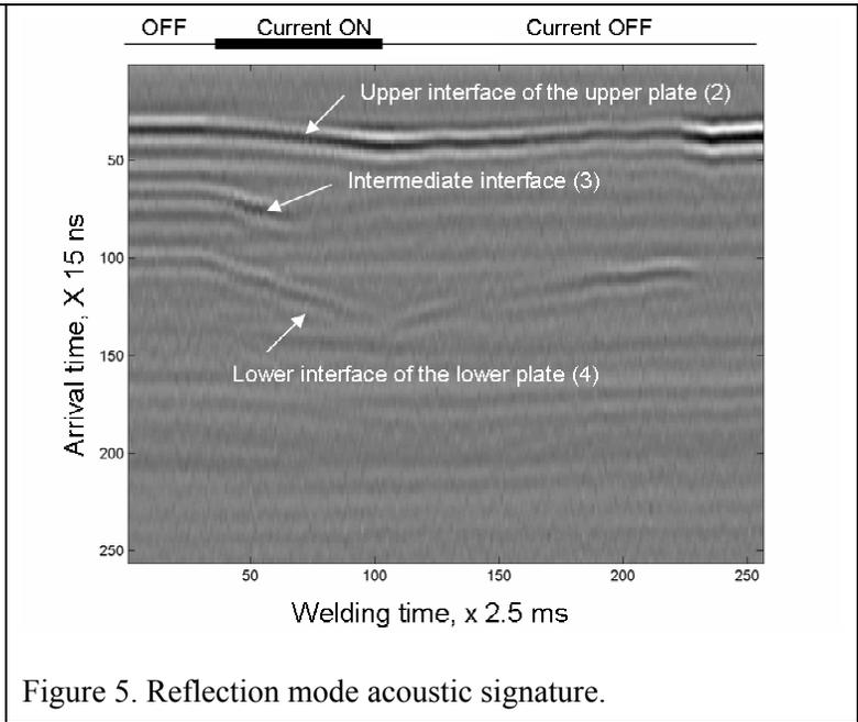
Figure 5. Reflection mode acoustic signature.
