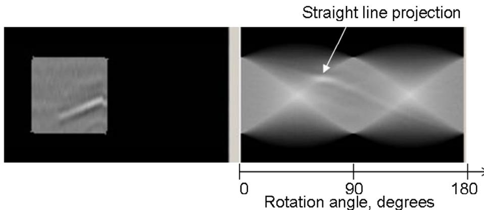
Figure 8. Image with line segment (left) and Radon transform image (right).
