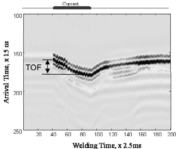
Figure 3. Signature of the spot weld. Through-transmission mode.
