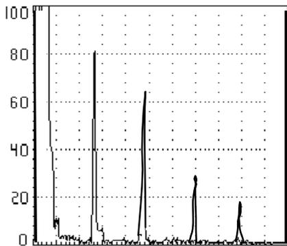
Figure 4 - Acceptable weld
