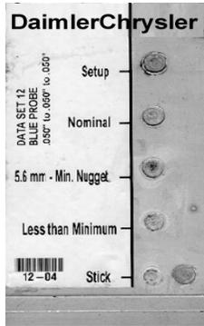
Figure 3 - Calibration Coupon
