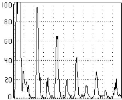
Figure 6 - Undersized weld
