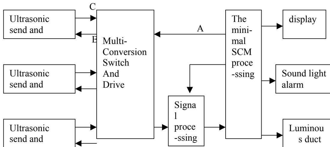
Figure 1: System hardware structural chart
