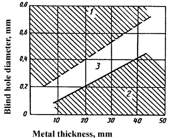
Fig. 4. The areas of 100% (1), zero (2) and  $(0 \leq P \leq 100\%)$  (3) probability of detection of drilled blind holes in aluminum in case of radiographic testing method.
