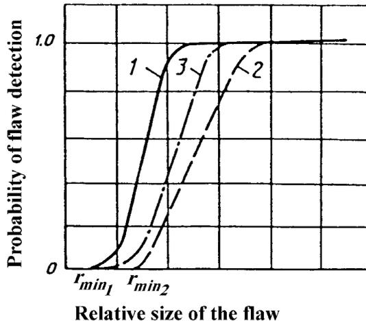
Fig. 3. Probability of flaws detection like a function of their sizes: curve 1 – experienced operator; curve 2 – non-trained operator; 3 – relationship described by equation (1).
