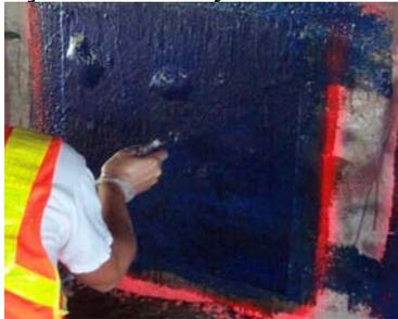
Figure 4. Intentional Delaminations on FRP Laminates.
