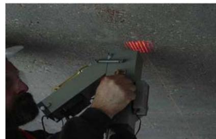
b) Roughness Detection by Laser Profilometer
