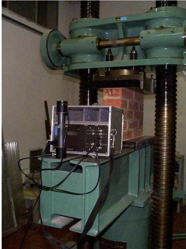
Figure 1. Preparation of the masonry panel for breaking test after having obtained the ultrasonic velocity data
