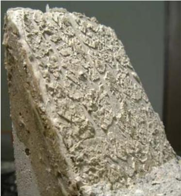
Fig.8 Fracture surface in the crack repair division.
