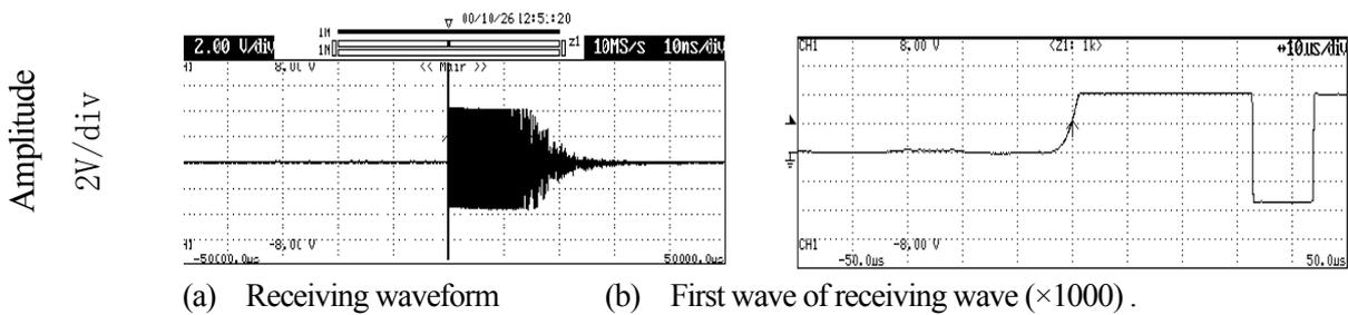
Fig.2 Waveform of soundness divisions in the concrete.
