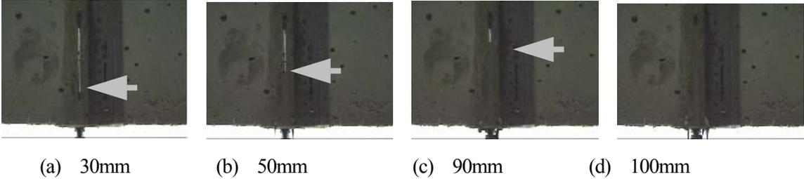
Fig.6 Injection situation of repairing materials
