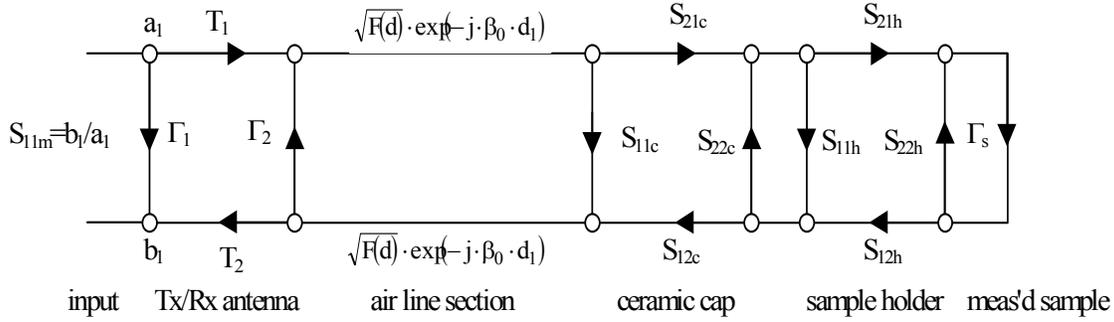
Figure 2. Signal flow graph model for the DCS.
