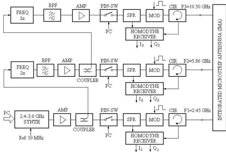
Figure 6. Block diagram of the microwave DCS for use in bins of raw materials and in concrete mixers.
