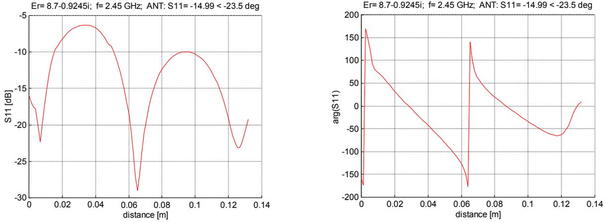
Figure 3. Simulation of the input complex reflection coefficient for moist sand versus d1 distance.
