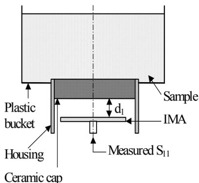
Figure 1. Cross- section view of the DCS.
