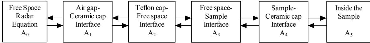
Figure 5. Double-path attenuation process for NCS.
