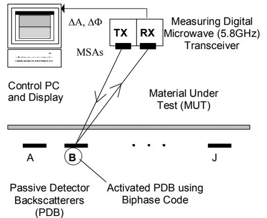
Figure 7. The basic measurement set-up for PBM (particle-board monitoring system).
