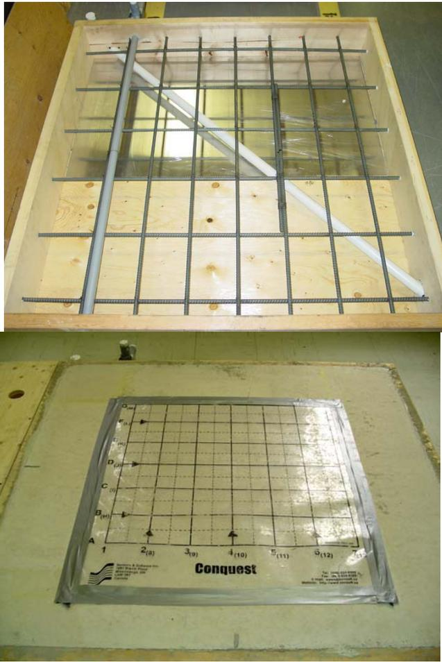
Figure 1: Test pad construction prior to concrete pour.
