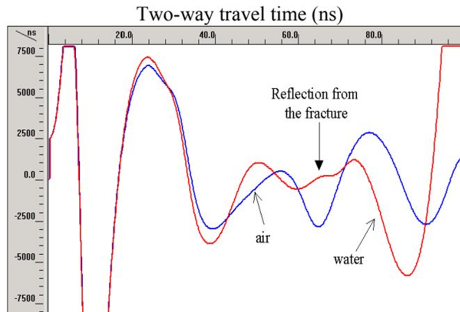
Figure 4 : GPR reflections on a water and air filled crack of 0.5 mm thickness
