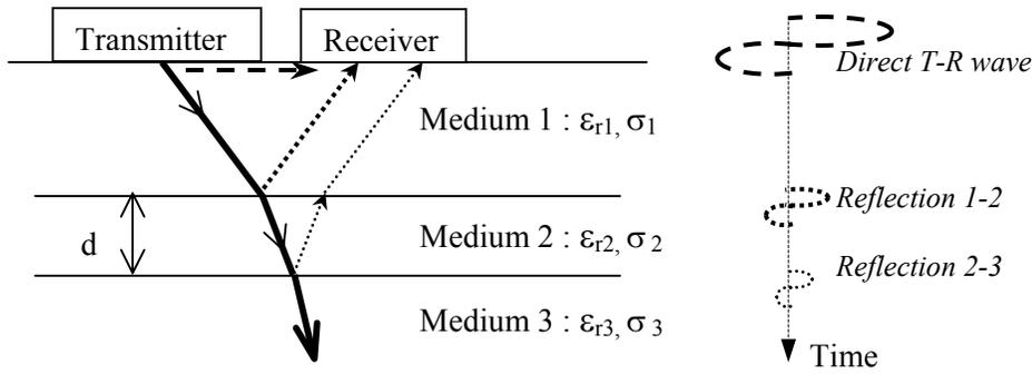
Figure 1 : Reflection and transmission of electromagnetic waves at interfaces
