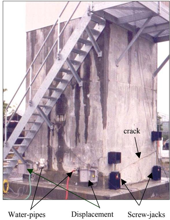
Figure 3 : External Instrumentation of the bloc
