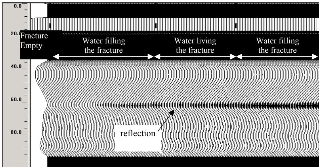
Figure 5 : GPR data obtained on a crack of 2 mm thickness
