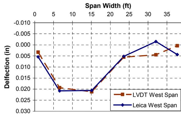
Figure 11: Stop 2 – West Span Deflection
