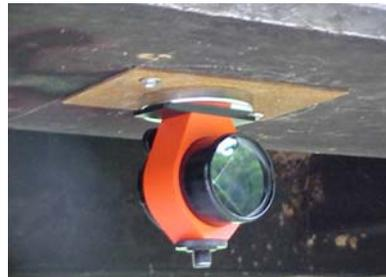
Figure 3: Target (Prism) on a bridge
