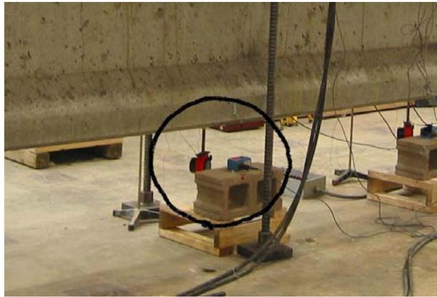
Figure 13: String Transducer and Mounted Prism
