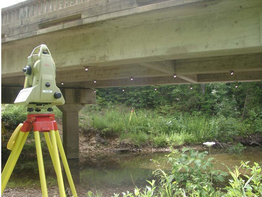
Figure 1: Leica TCA 2003 set up for Load Testing
