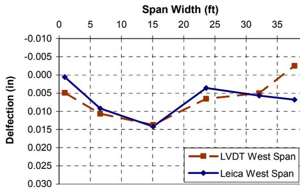
Figure 10: Stop 1 – West Span Deflection
