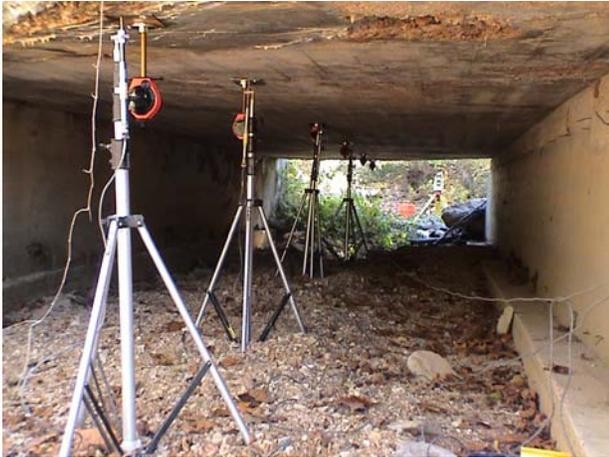
Figure 8: LVDT's and Prisms
