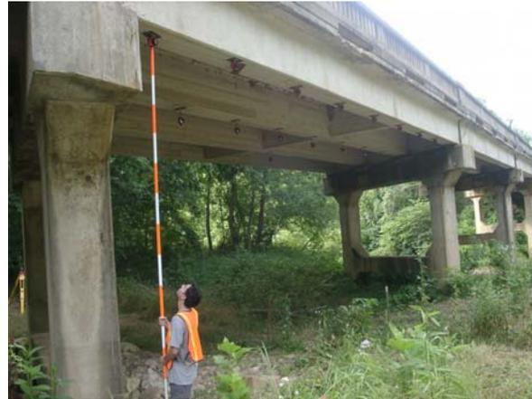
Figure 7: Mounting the Targets
