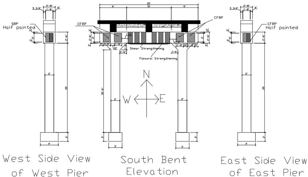
Figure 4. South side view of south bent
