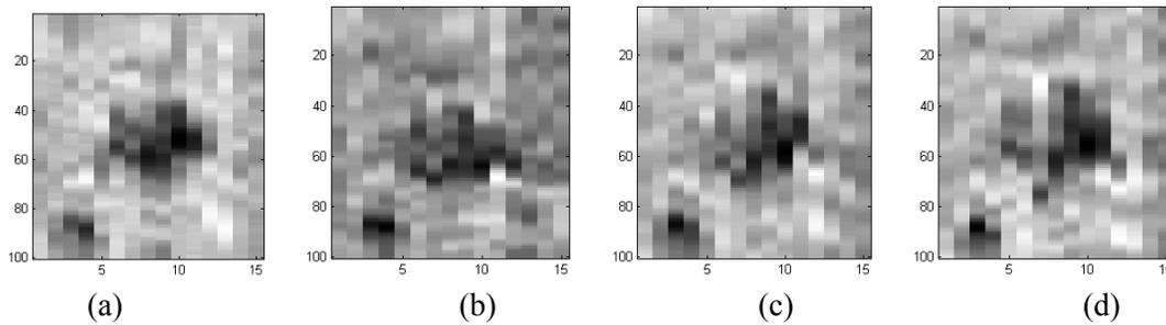
Figure 8. Image of the delamination in Figure 1 under perpendicular polarization. (a) before cycling, (b) after 500K cycles, (c) after 1-million cycles and (d) after 2-million cycles.
