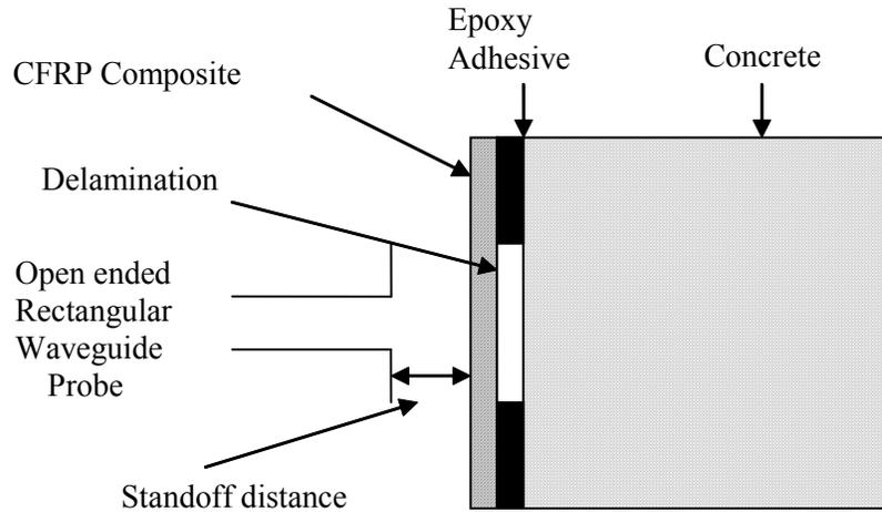
Figure 4. Schematic of a near-field microwave measurement system.
