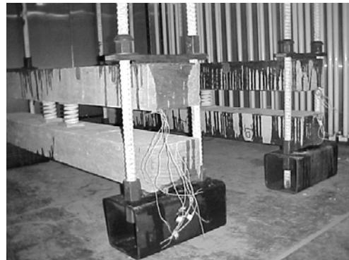
Figure 2. Test beam with delaminations. Figure 3. Environmental conditioning of beams.
