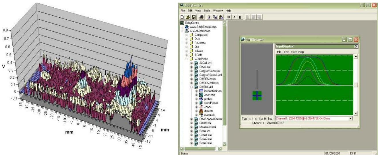
Figure 5 – Measured data in differential mode with 3 semi-elliptical slots and modeled central line scans over 6 defects
