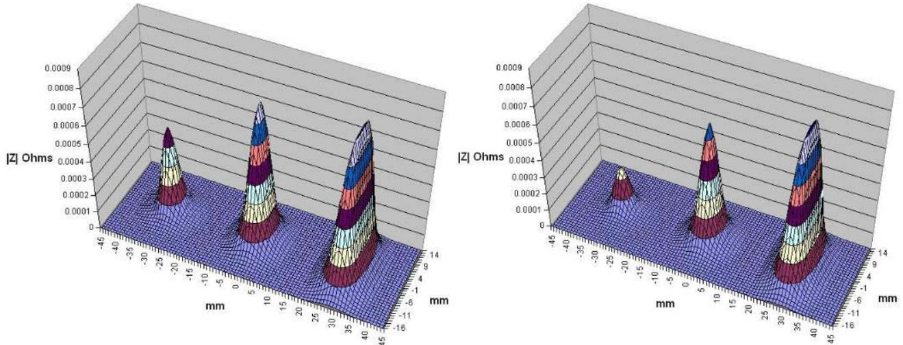
Figure 6 – Differential mode: rectangular and semi-elliptical slots
