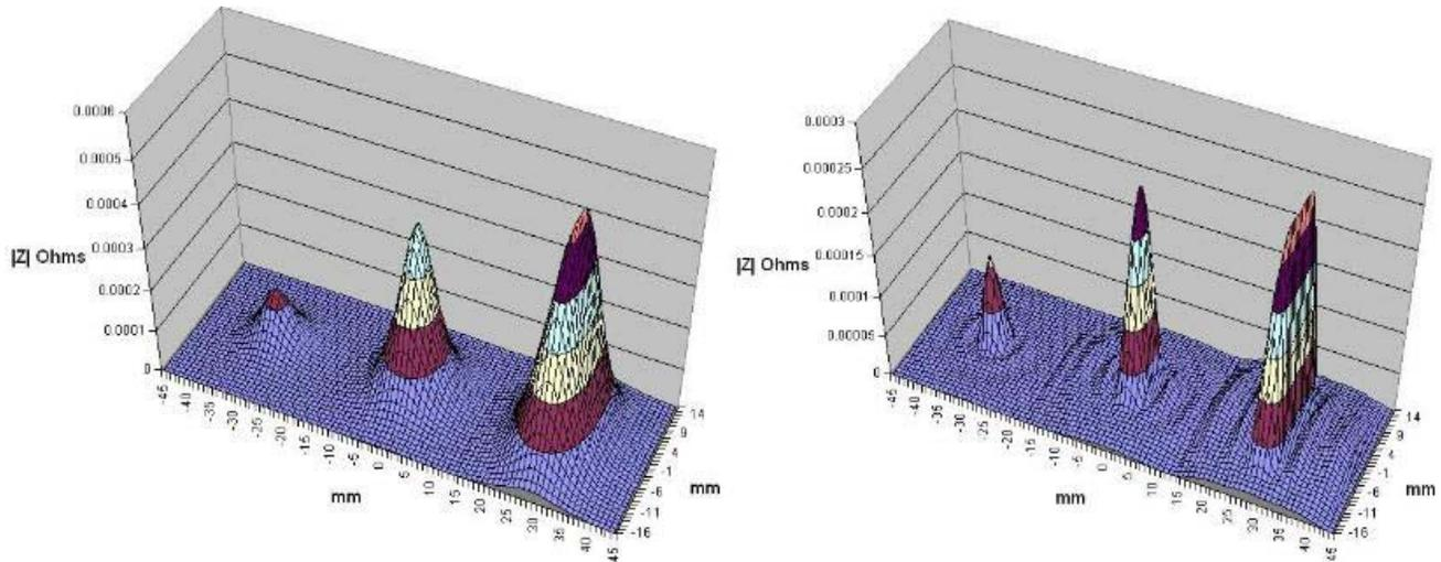
Figure 4 – Absolute mode: 3 semi-elliptical slots 0.1x5x0.5, 0.1x10x1 and 0.1x20x2 mm
