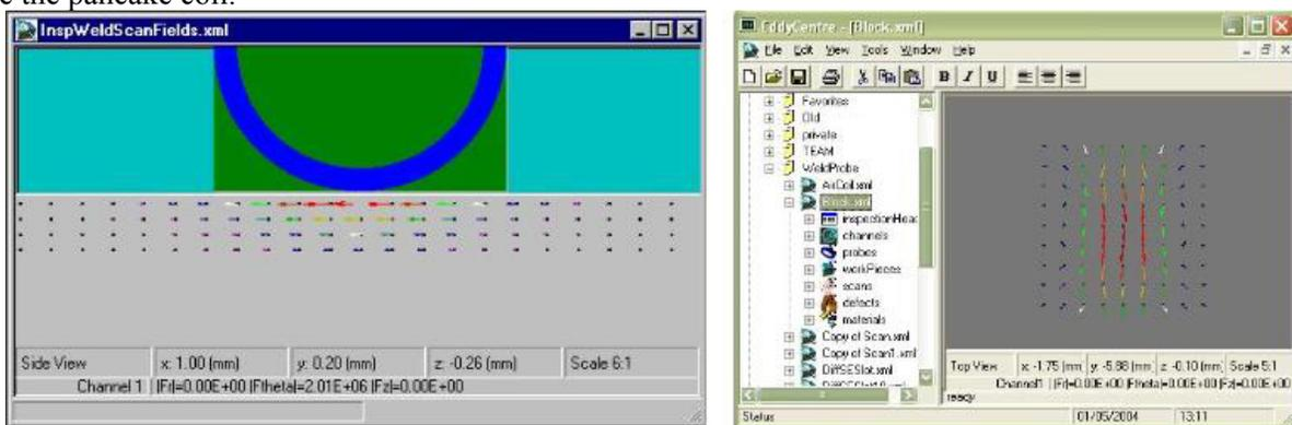
Figure 1 - Tangential coil and associated electric field inside an aluminum block
