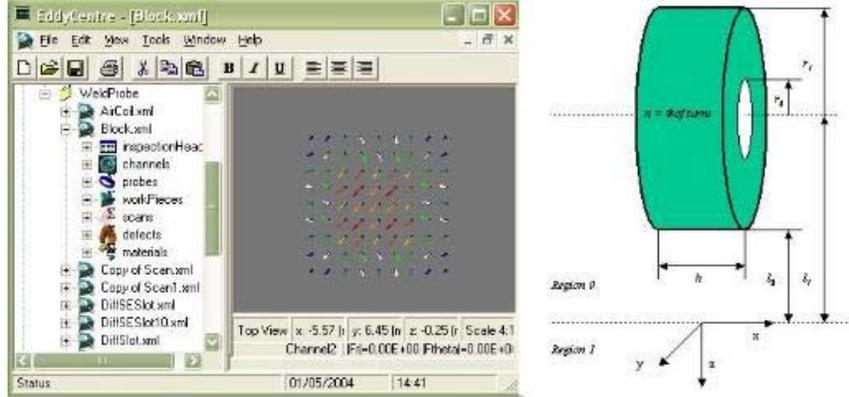
Figure 2 -Fields from 2 interwoven tangential coils and coil parameters
