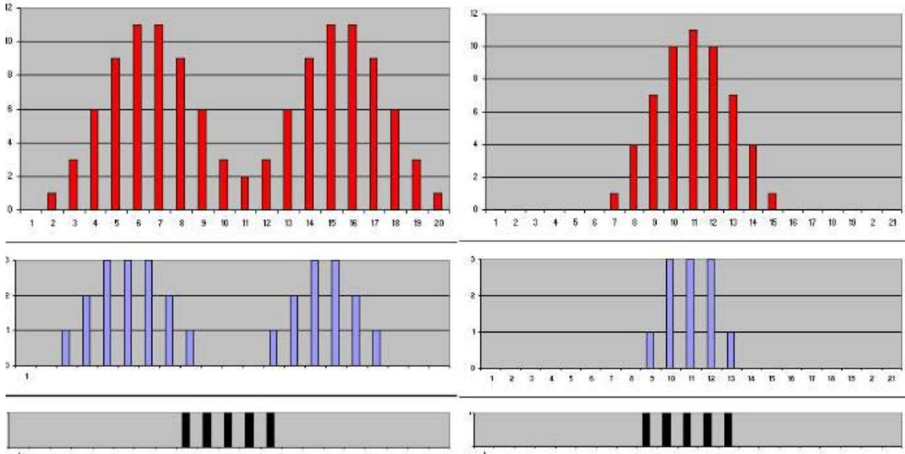
**Figure 7 – defect, probe field (pancake and tangential) and eddy-current (convolved) signals**
