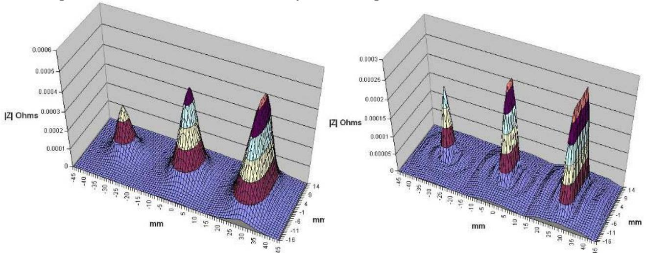
Figure 3 – Absolute mode: 3 rectangular slots 0.1x5x0.5, 0.1x10x1 and 0.1x20x2 mm
