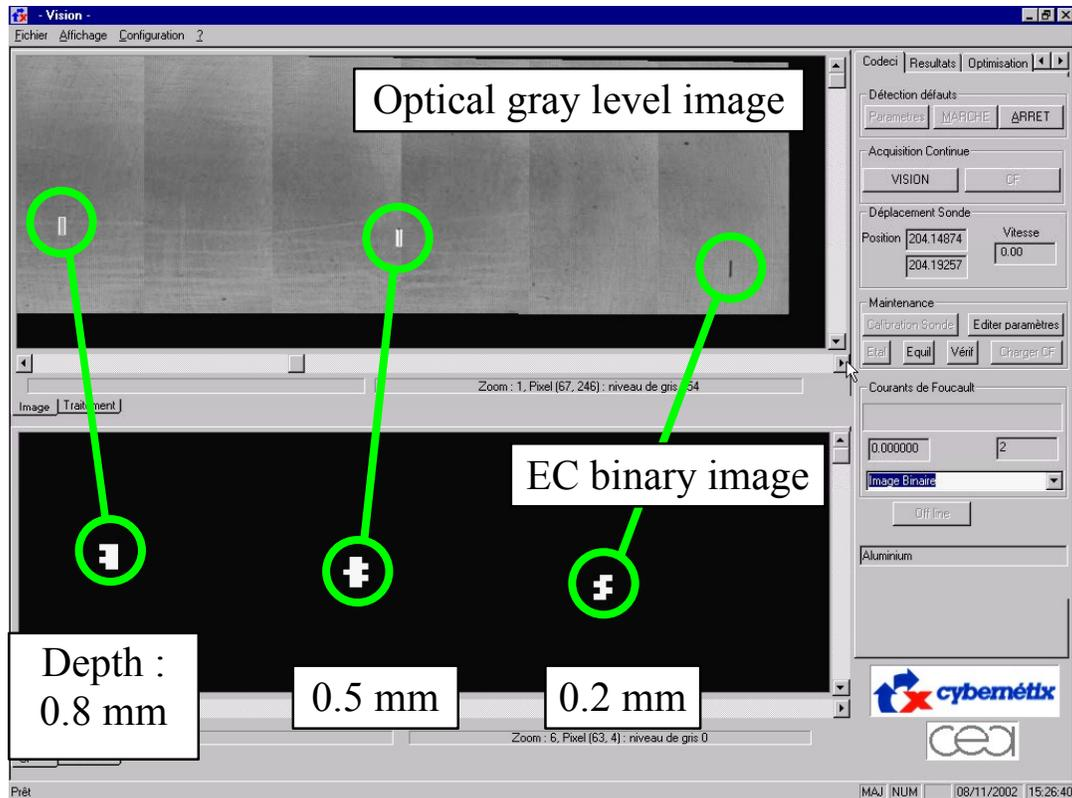
Figure 5: Detection and characterization of notches of 1 mm long in an aluminium slab.
