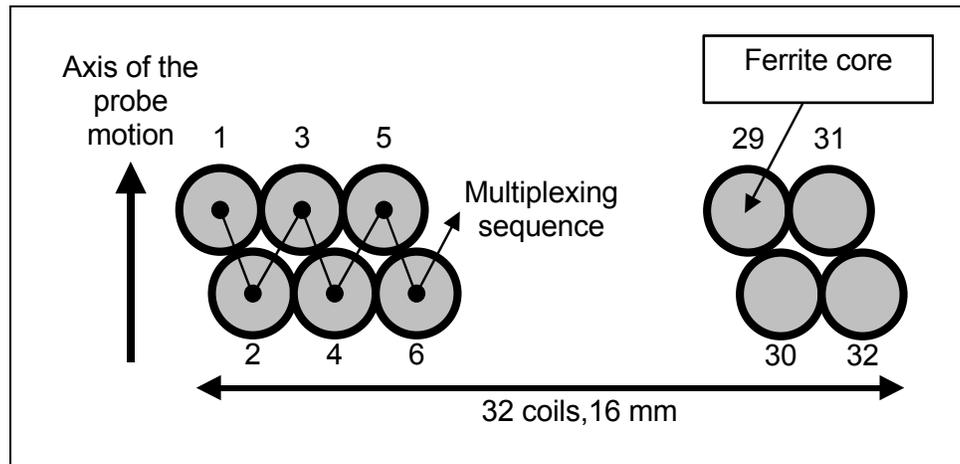
Figure 3: Eddy current array probe and multiplexing sequence.
