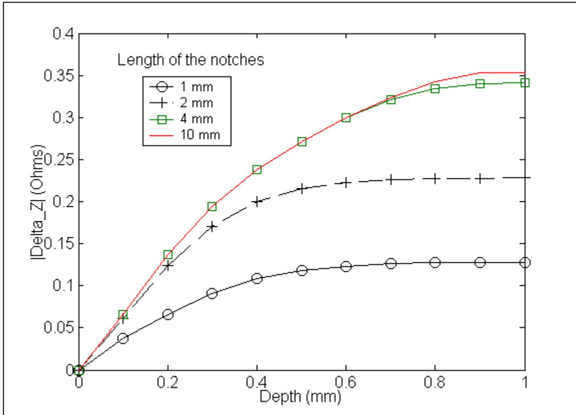
Figure 4: Maximum of the variation of the coil impedance for a rectangular EDM notch.
