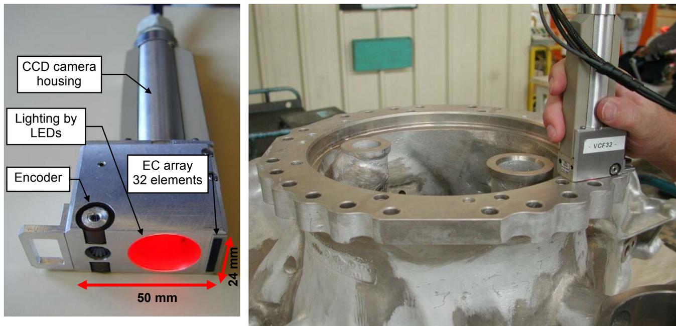
Figure 2: General view of the CODECI probe. Inspection of an helicopter gear housing with the probe.
