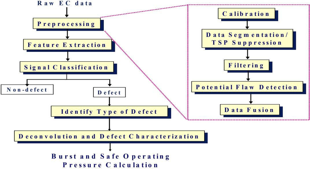
Figure 2. Eddy Current Data Analysis System.
