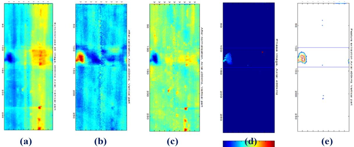
**Figure 3. Results at various stages of preprocessing (a) Raw data (b) calibration (c) TSP suppression (d) thresholding (e) data fusion and potential flaw identification.**
