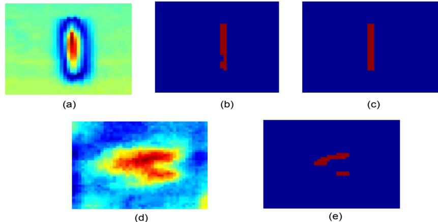
**Figure 5. Deconvolution (a) original signal (b) flaw footprint for signal in (a) after deconvolution (c) actual flaw footprint (d) example of measurement from multiple flaws in close proximity (e) separation of multiple flaws after deconvolution.**
