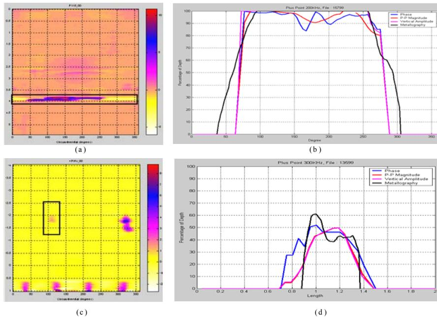
**Figure 4. Flaw profiling: (a) Circumferential Defect (b) estimated and true flaw profile (c) axial flaw (d) estimated flaw profile.**
