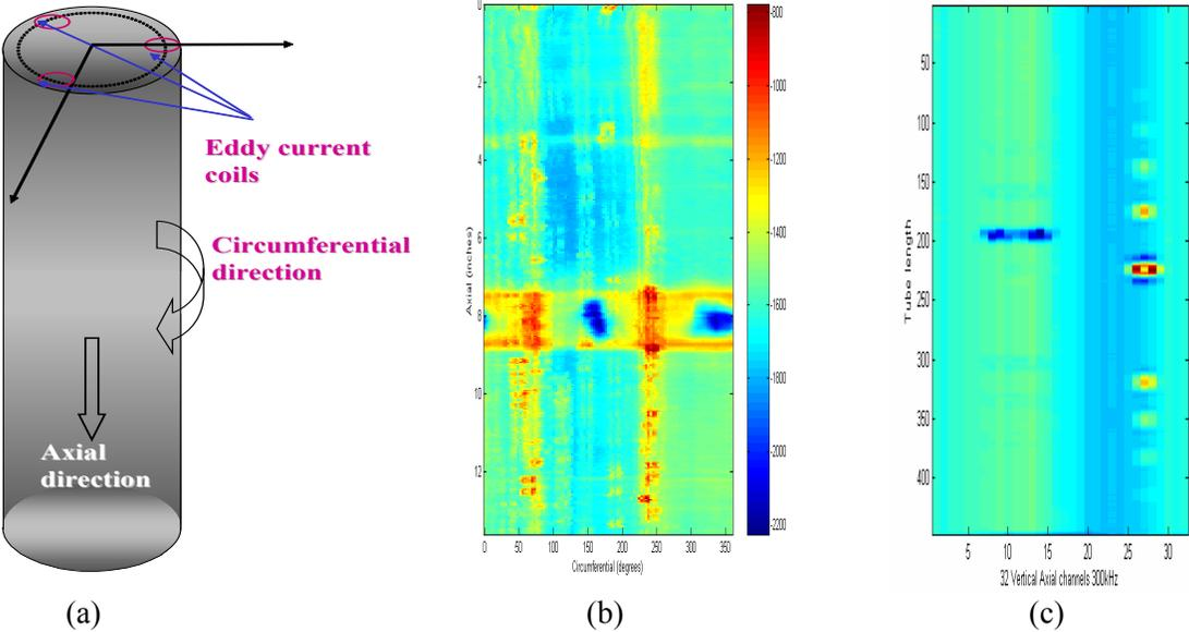
Figure 1. (a) RPC configuration (b) Typical RPC data (c) Typical Array probe data.
