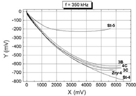
Figure 6. Resistivity assessments on the Zircaloy-4 samples with different hydrogen content and on as-received Zircaloy-4, two-layer coil 1.
