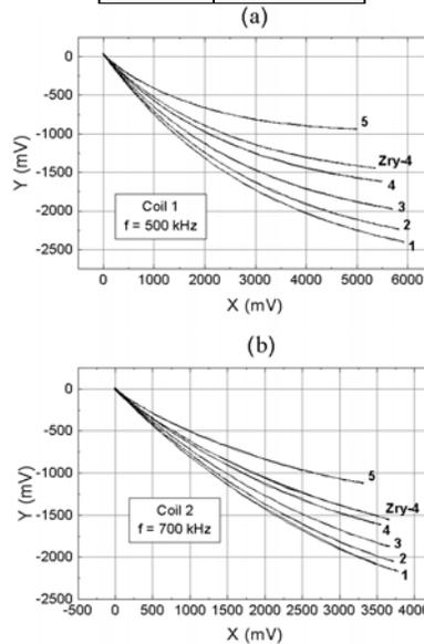
Figure 5. Material sorting tests on the resistivity standard set and the Zircaloy-4 block: (a) two-layer probe 1, (b) single-layer probe 2.
