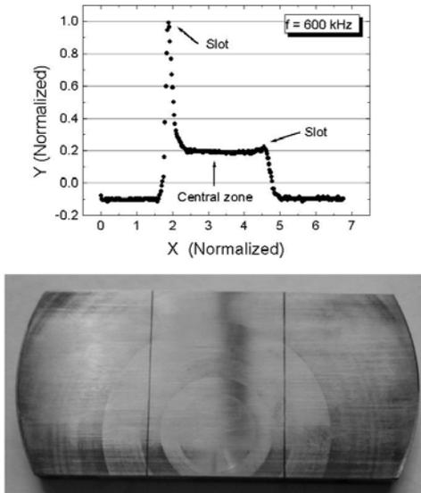
Figure 2. Tool marks on the surface of one of the Zircaloy-4 blocks used for the inspection of surface defects, and the  $x(t)$  component of one signal showing the unbalance of the bridge, which is a consequence of these surface imperfections.
