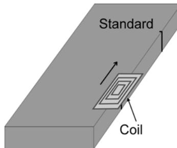
Figure 4. Balance technique for edge defect detection.
