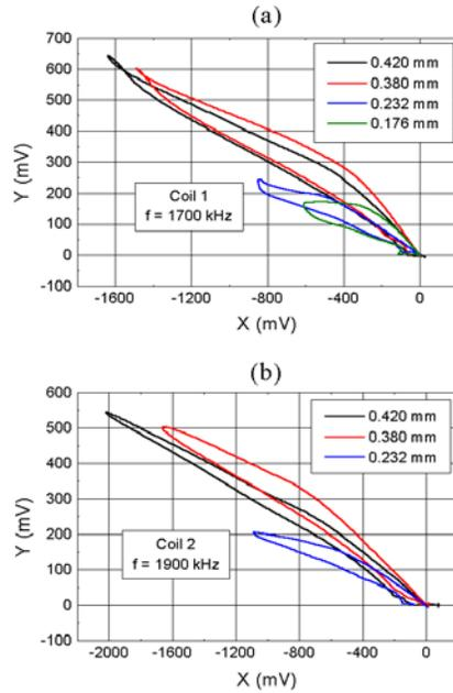
Figure 1. Signals obtained during the inspection of surface defects with two-layer coil 1 and single layer coil 2 at different inspection frequencies.
