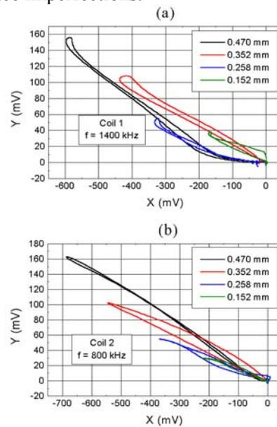
Figure 3. (a) Results from inspections of edge cracks with two-layer coil 1 at 1400 kHz of operation frequency, (b) results for single layer coil 2 at 800 kHz.
