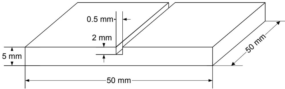
**Figure 3 Aluminium Testing Sample with a Surface Slot**
