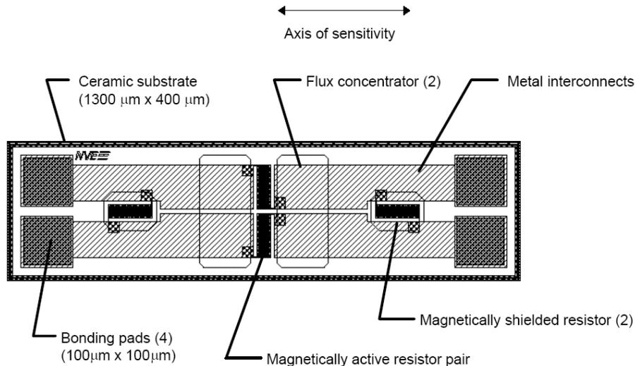
**Figure 1 Typical GMR sensor layout**
