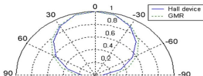
**Figure 2 Polar Plot of Normalised Output vs. Angle of Magnetic Field**
