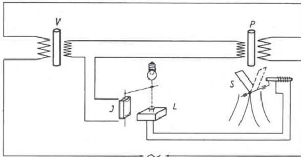
Figure 1: Schematic Diagram of an Early Eddy Current System Developed by Förster [2]
