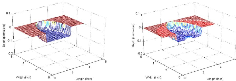
Figure 4: True and Reconstructed Defect Profiles Obtained From Magnetic Flux Leakage Signals Using Wavelet Functions
