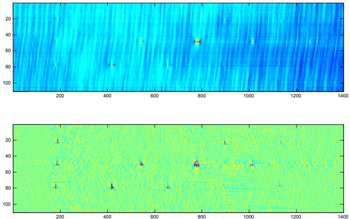
Figure 3: Original (top) and Filtered Magnetic Flux Leakage Images.
