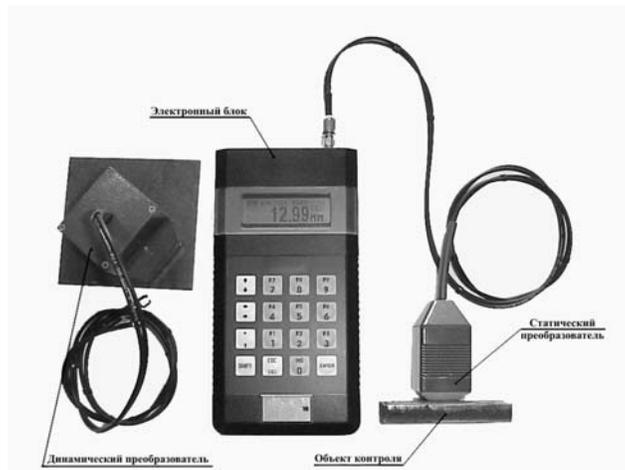
**Fig. 4.** Ultra-sound thickness gauge EMAT-100
