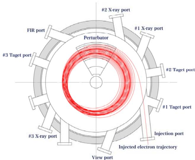
MIRRORCLE-6X accommodates 3 x-ray beam ports as seen in Fig. 2. The beam trajectory is illustrated in red colour. Each port is assigned to X-ray crystallography, X-ray microscope, X-ray fluorescent analysis, and X-ray imaging. The X-ray microscope and X-ray crystallography beam line is equipped with a focusing element made of multi-layered set of 8, concentrically aligned, cylindrical mirrors.
