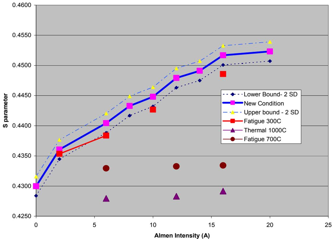
Figure 5. Thermal and Fatigue Effects as Compared to Original CMSX-4 Shot Peened Samples
