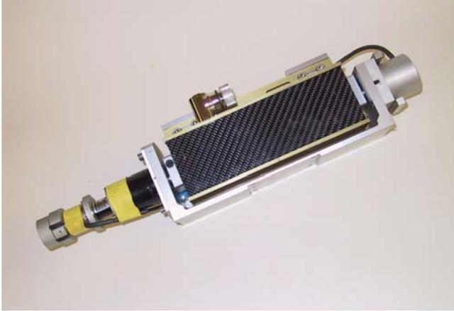
**Fig. 4:** View of the line camera system, mounted in the manipulation holder. The line camera contains two CMOS-lines and a double slit collimator in front of the lines. The size amounts 200mm x 70mm x 40mm. (manufactured by NTB elektronische Geräte GmbH, Dickel, Germany)
