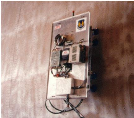
**FIGURE 1:** MACS crawling on the C-5 aircraft [Bar -Cohen, 2000].
