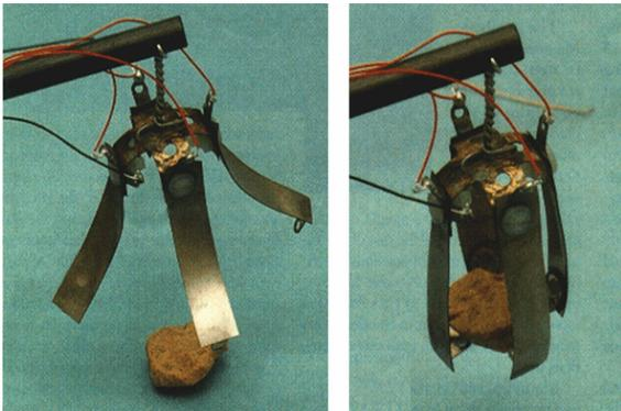
**FIGURE 3:** 4-finger EAP gripper lifting a rock.
