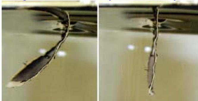
**FIGURE 7:** Conductive EAP actuator is shown bending under stimulation of 2-V, 50-A.
