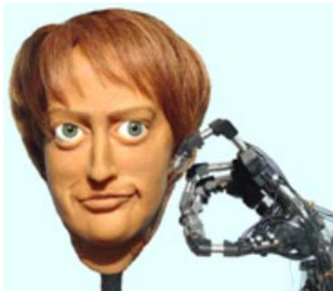
**FIGURE 8:** An android head and a robotic hand that are serving as platforms for the development of artificial muscles [This photo was made at JPL where the head was sculptured and instrumented by D. Hanson, University of Texas, Dallas. The hand was made by G. Whiteley, Sheffield Hallam U., UK.]
