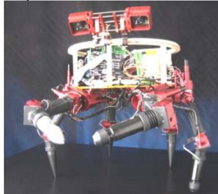
**FIGURE 2:** A new class of multi-limbed robots called LEMUR (Limbed Excursion Mobile Utility Robot) is under development at JPL [Courtesy of Brett Kennedy, JPL]
