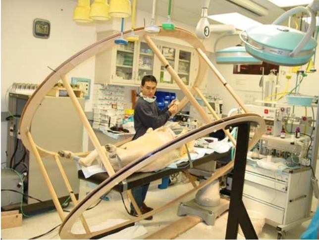
Figure 4: Excitation Coil Assembly and the Surgery Table
