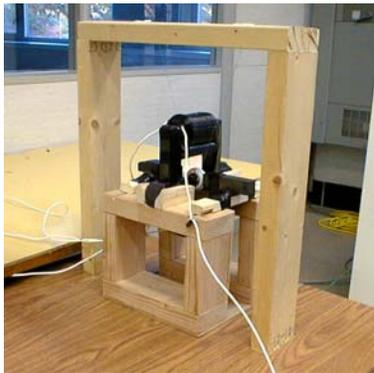
Figure 11: EMAT system for demonstrating proof of concept
