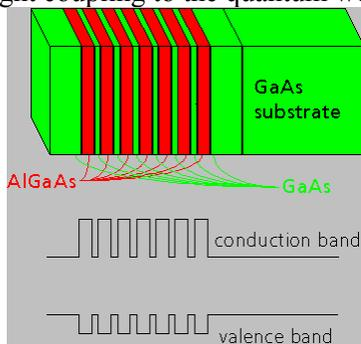
Figure 6: Schematic of epitaxial GaAs/AlGaAs quantum well layers on a GaAs substrate and resulting band-edge distributions
