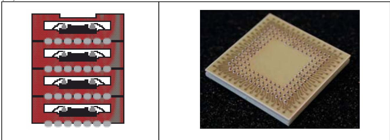
Figure 9: Principle design of a Match-X-system (left: with 4 components) and design of a single component (right).
