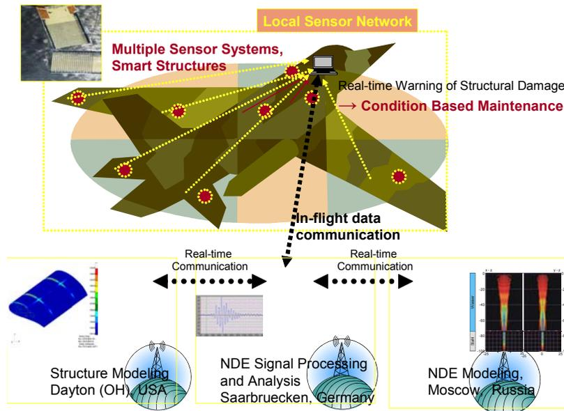
Figure 11: Concept for continuous health-monitoring of aircraft while in use
