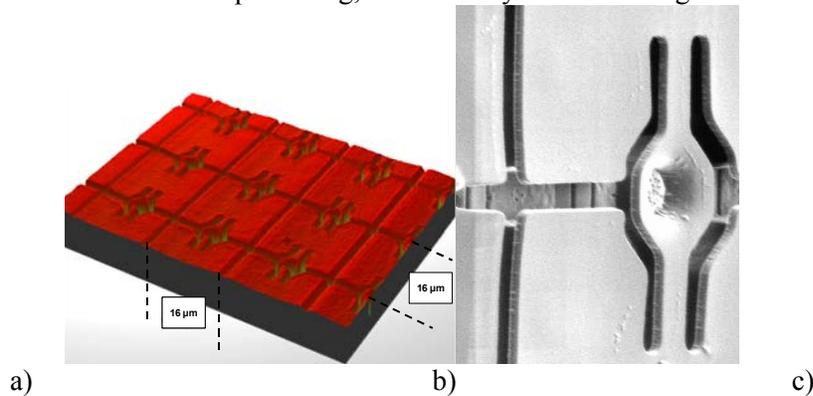
Figure 4: Micro-mirror-chip in ceramic frame (a), white light interferometer image of the mirror array (b) and FIB (focused ion beam) image of an Al-blade at the hinge section (c).
