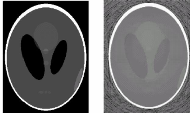
Figure 8: Reconstruction of the Shepp-Logan phantom. Left: rasterized phantom, right: reconstruction results (9).
