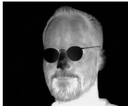
Figure 7: Image taken with a 512 x 640 pixel high-resolution thermal imaging-camera with only 7mK noise (8)
