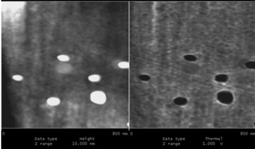
Figure 2: AFM (left) and UFM (right) images of nano-precipitations in Al 7075-T6 [4].
