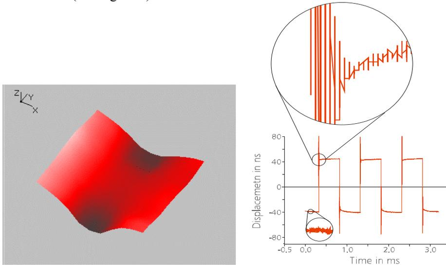
Figure 5: Butterfly mode (868 kHz, left) and short-time switching behavior (right) of an individual mirror blade detected by the Laser vibrometric microscopy.
