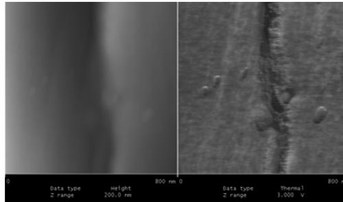
Figure 3: AFM (left) and UFM (right) images of interaction of a crack and nano-precipitations in Al 7075-T6. The crack path is modified by the two large precipitations [4].
