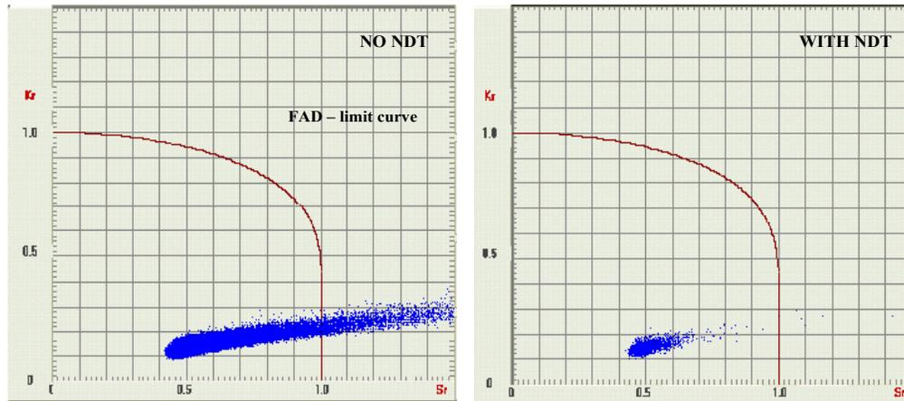
Figure 10: Effect of NDT on risk failure at 10.000 load cycles in a riveted joint (Al-alloy).
