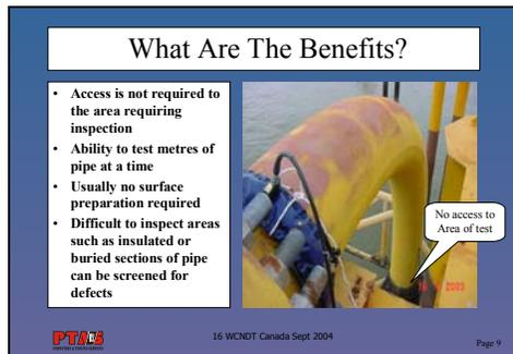
Access is not required to the area requiring inspection, it has the ability to test many metres of the riser at one time. Usually no surface preparation is required. Difficult to inspect areas such as splash zone or buried sections of the riser can be inspected.
