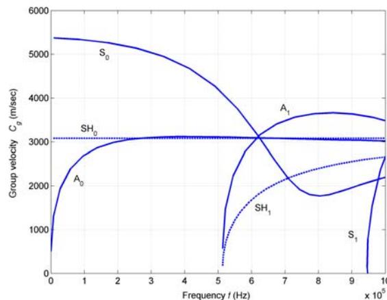
Figure 2 The group velocity – frequency relation of the guided waves in a 3 mm thick aluminum plate.
