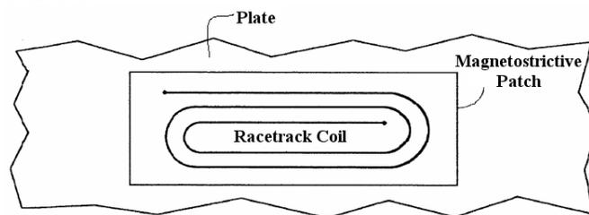
Figure 1 The patch-type magnetostrictive transducer by Light *et al.*<sup>9</sup>
