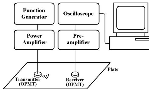
Figure 4 Schematic diagram of the experimental arrangement. (Function generator: Agilent 33120A, Power Amplifier: RAM5000, Pre-amplifier: SR560 , Oscilloscope: Lecroy LT354 )
