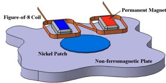
Figure 3 Schematic diagram of an OPMT
