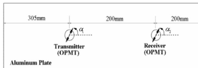
Figure 5 Experimental setup for guided wave generation and measurement by OPMT. The arrows denote the direction of the applied bias magnetic flux.
