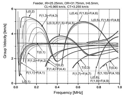
Fig. 2 Phase velocity dispersion curve for the feeder.
