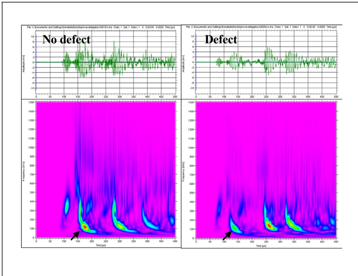
**Figure 10.** Lamb wave signal changes due to presence of skin crack. The wavelet modal analysis diagrams show a loss of energy in lower frequency mode and corresponding ultrasonic energy shift to higher modes when crack discontinuity is present in the sample. An arrow highlights the lower mode in the diagrams. Horizontal axes represent relative time and vertical axis frequency.
