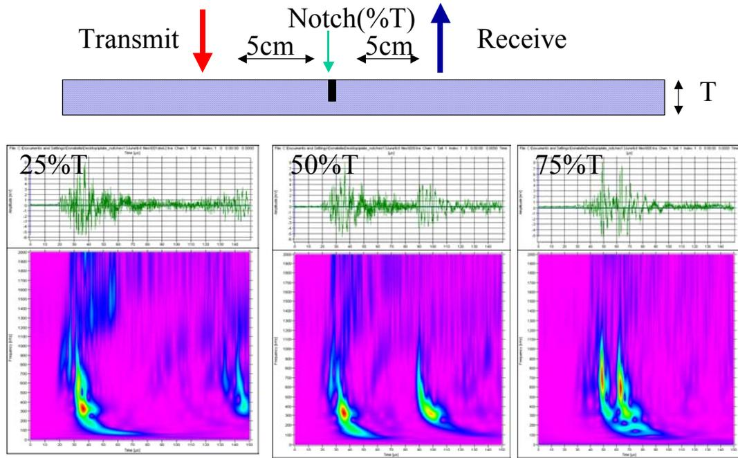
**Figure 11.** Ultrasonic signal amplitude transmission level for different depth of the notch (crack) in plate with thickness T. The wavelet diagrams show significant shifts in modes and mode energy that are influenced by presence of crack like discontinuity. The results indicate the ability to analytically estimate crack depth using the wavelet signal analysis information
