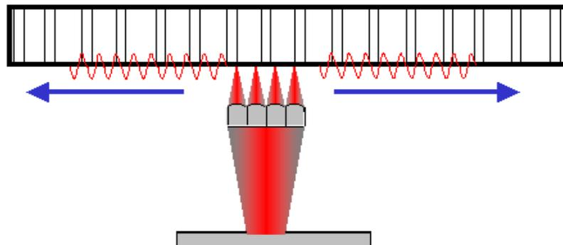
**Figure 5.** Controlled frequency laser ultrasonic set up for testing large area honeycomb panels .
