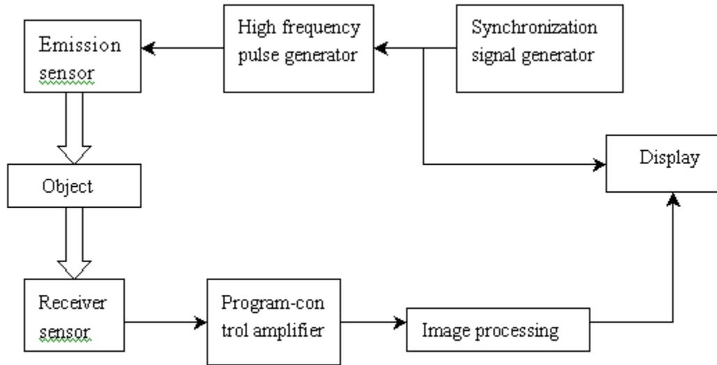
Figure 1. Transmitted Ultrasonic Imaging System
