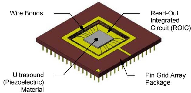
Figure 2. Array Schematic
