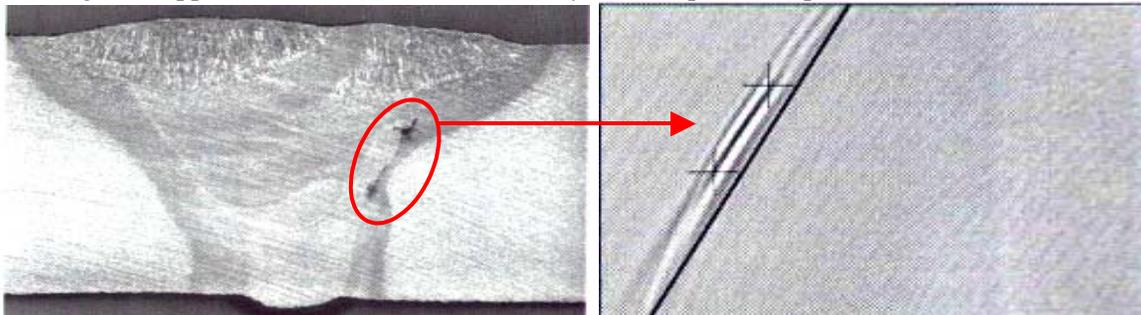
figure 5: Multi SAFT image (right) showing the result of a lack of fusion defect (left). Courtesy Maarten Lorenz (Shell Global Solutions International).
