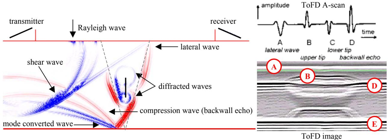
figure 4: Elastic finite difference simulation of the ToFD principle, showing all the important events: A) lateral wave, B) diffraction of the upper defect tip, C) diffraction of the lower defect tip, D) reflection at the back wall, E) signal caused by the mode converted wave.
