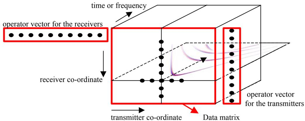
figure 1: Three dimensional data matrix for all transmitter and receiver combinations. The vectors  $V_s$  and  $V_r$  operate on a slice of the data matrix.
