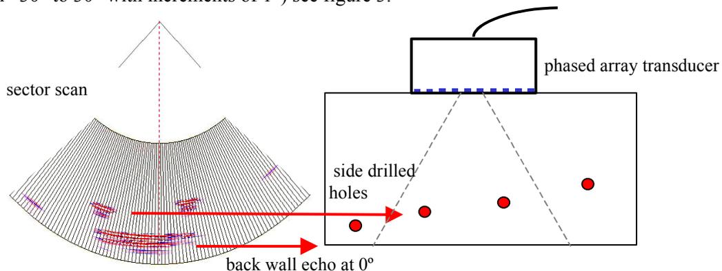
figure 3: Sector scan made on a block with side drilled holes.
