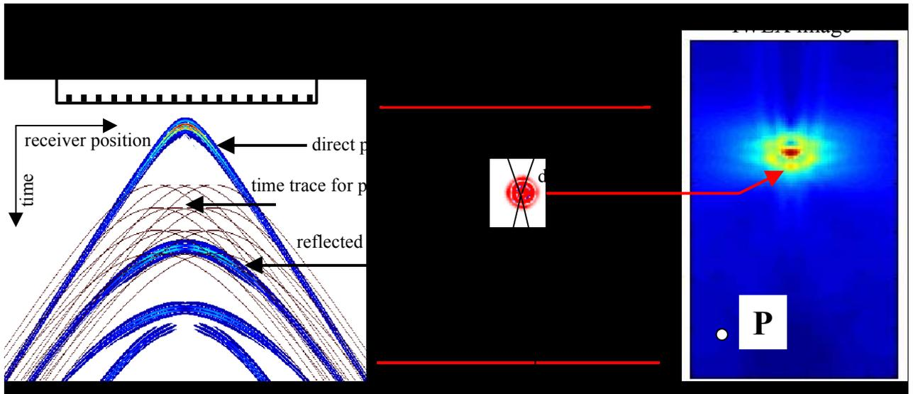
figure 2: (left) Response (simulated) caused by a cylindrical reflector, the reflector is assumed to be a source. (centre) Possible paths from the reflector (red dot) to the receivers. (right) Result of the IWEX image, when all points in the area are imaged. Point P does not contribute to the image, because no corresponding values can be found in the data at the left.
