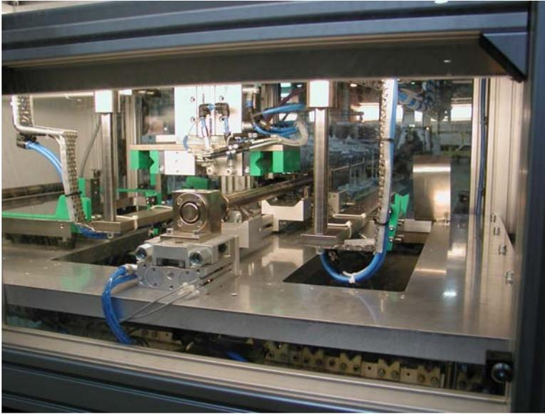
Figure 8: Automatic resonance testing of steering racks
