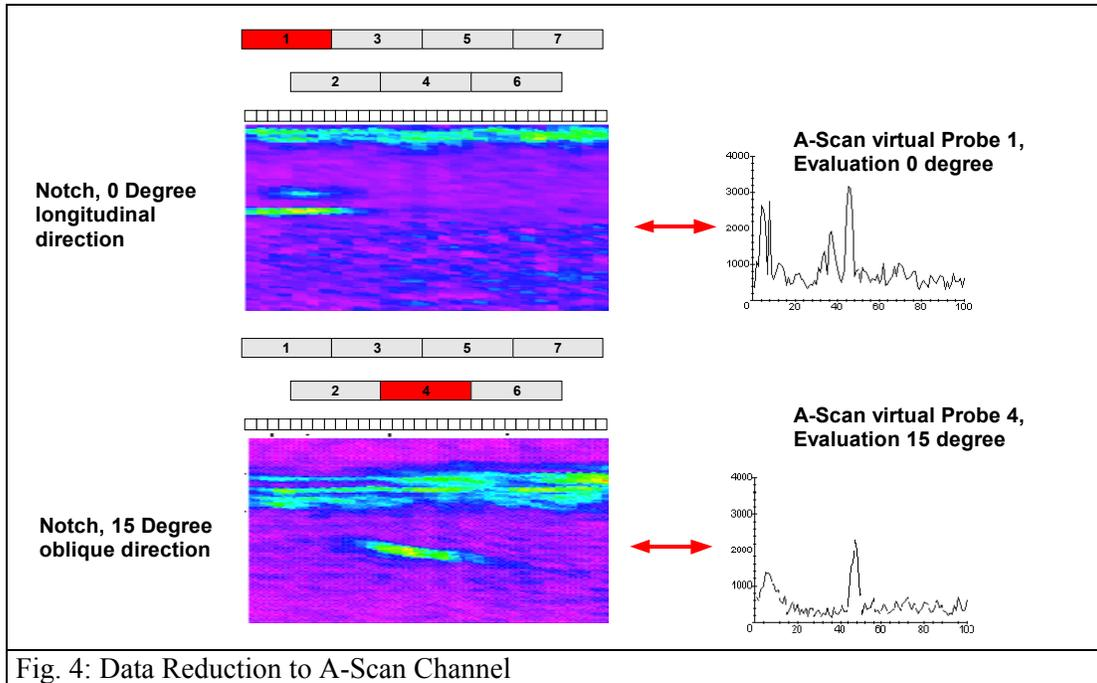
Fig. 4: Data Reduction to A-Scan Channel
