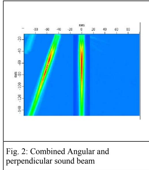
Fig. 2: Combined Angular and perpendicular sound beam
