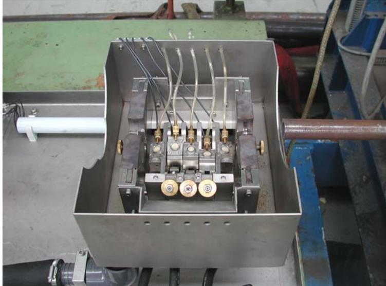
Fig. 3: Test tank of the tube end tester
