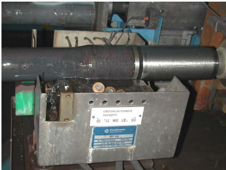
Fig. 4: Inspection of upset ends with REP-VIS
