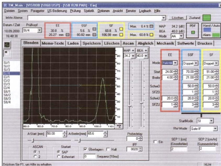
Fig. 5: Windows-based graphical user interface - Menu "Flaw test"
