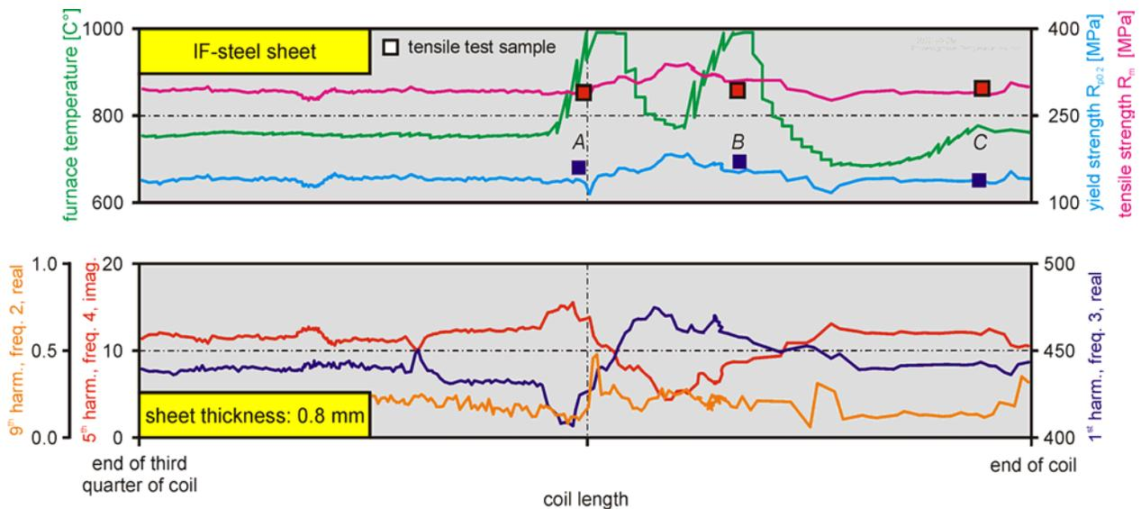
**Figure 5:** IF-steel sheet with a furnace temperature inconsistency
